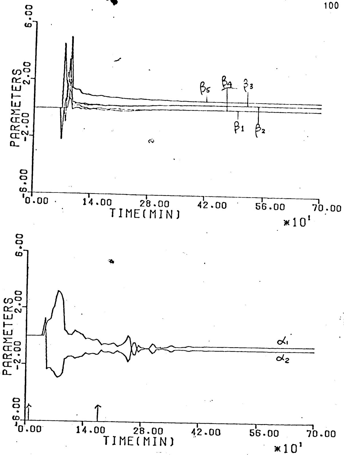
Figure 5.8 Adaption Pattern Of Parameters For a Pulse Disturbance In Feed Flow Rate Of -3.6 g/s In Magnitude For a Duration Of 170 Minutes, Starting With Zero Initial Parameter Estimates
