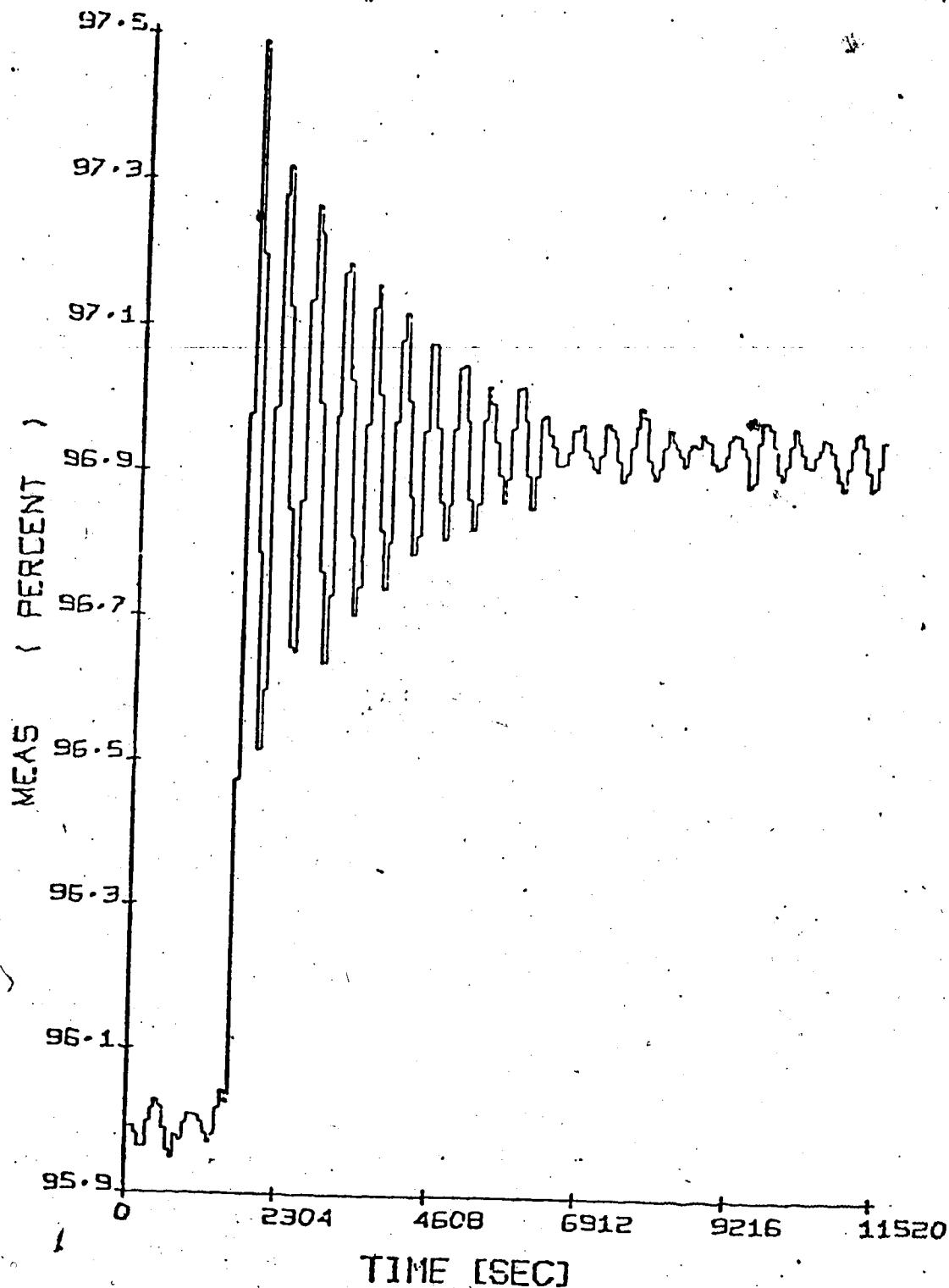
FIGURE D1 TOP PRODUCT COMPOSITION RESPONSE TO A +1% STEP CHANGE IN SET POINT USING A PROPORTIONAL CONTROLLER WITH  $K_p = -100.0$
