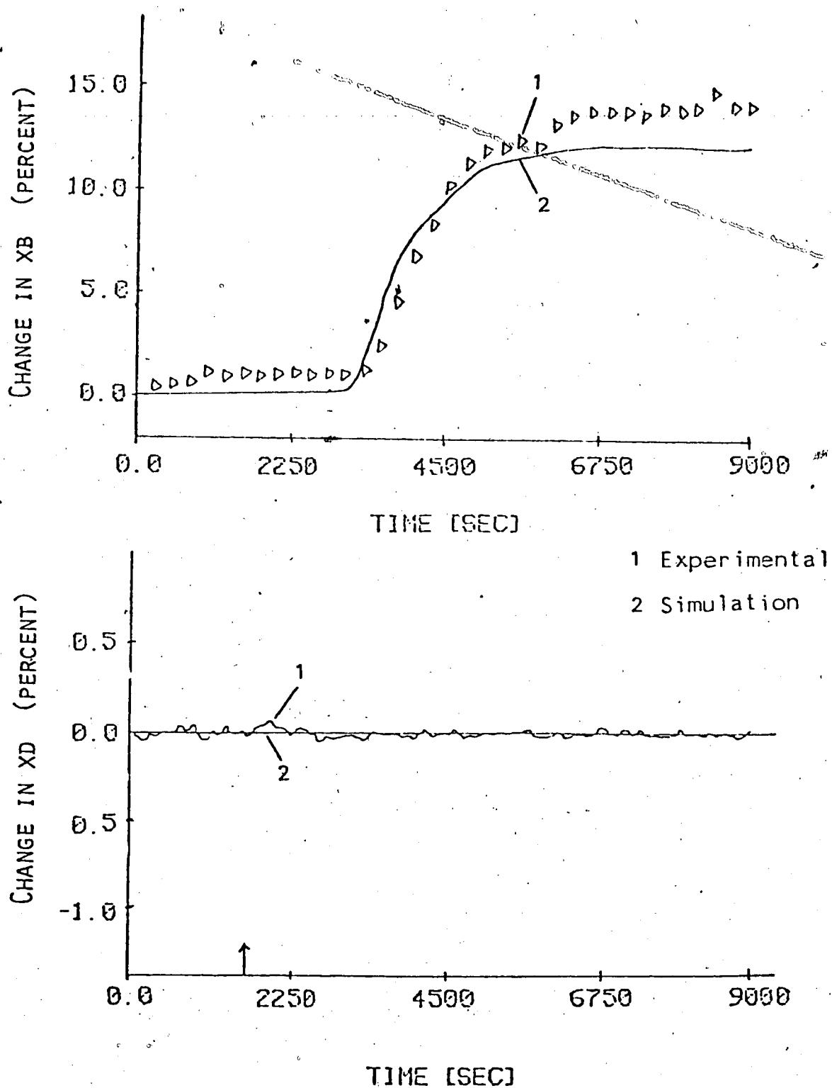
Figure 3.8 Comparison of Predicted and Experimental Dynamic Response of the Terminal Compositions to a Feed Flow Rate Step Change of + 20%
