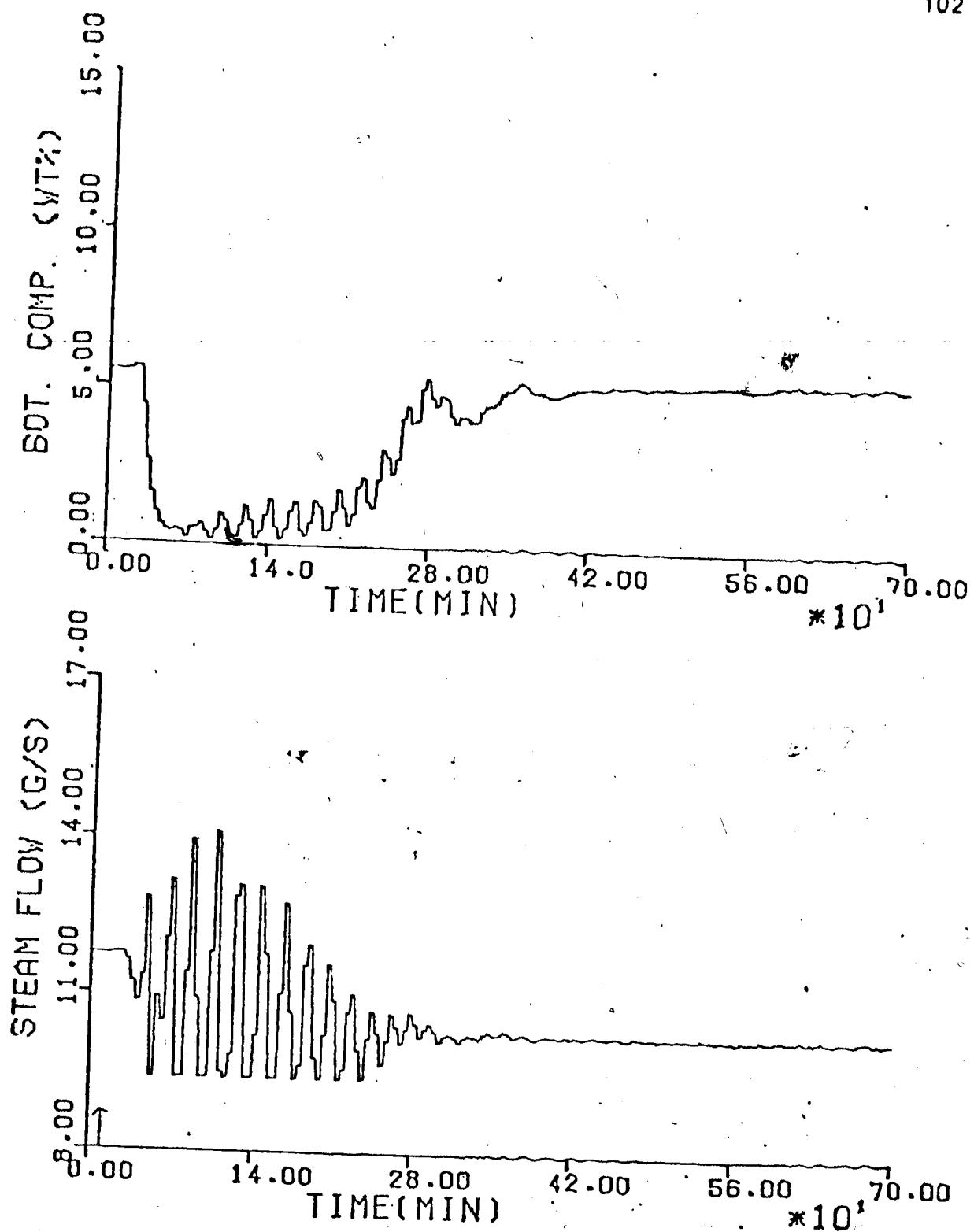
Figure 5.9 Simulated Response Of STR Bottom Product Composition Control For a -20% Step Change In Feed Flow Rate, Starting With The Initial Estimates As Those Obtained From Run B11
