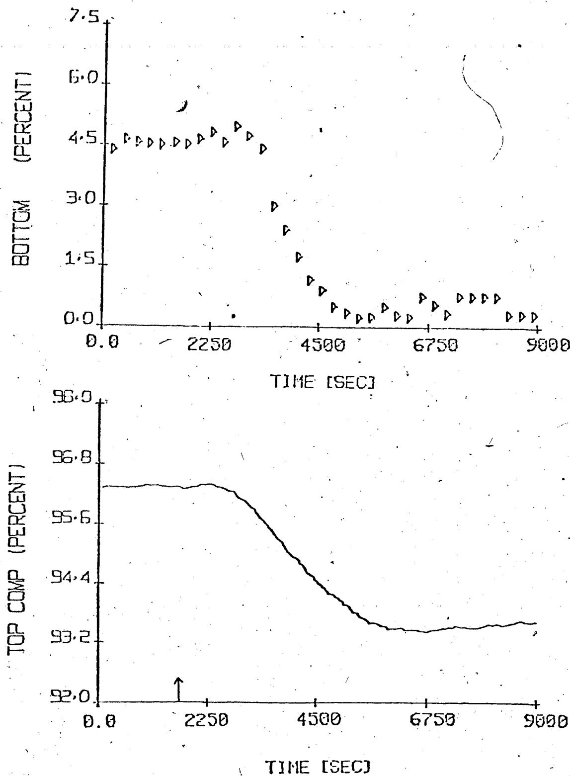
Figure 3.3 Dynamic Response of the Terminal Compositions to a Feed Flow Rate Step Change of -20%
