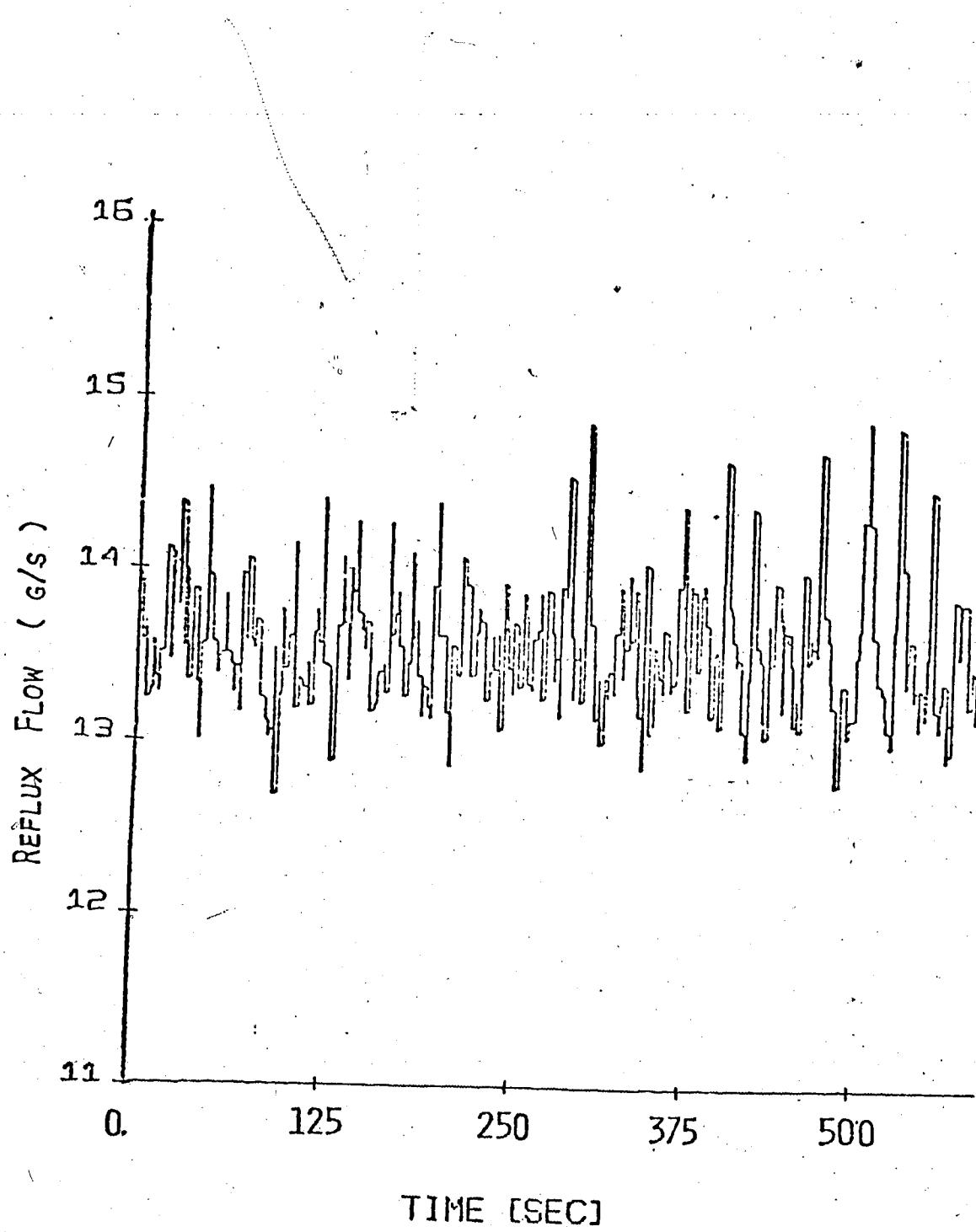
Figure 3.13 Experimental Steady State Reflux Flow Noise Display
