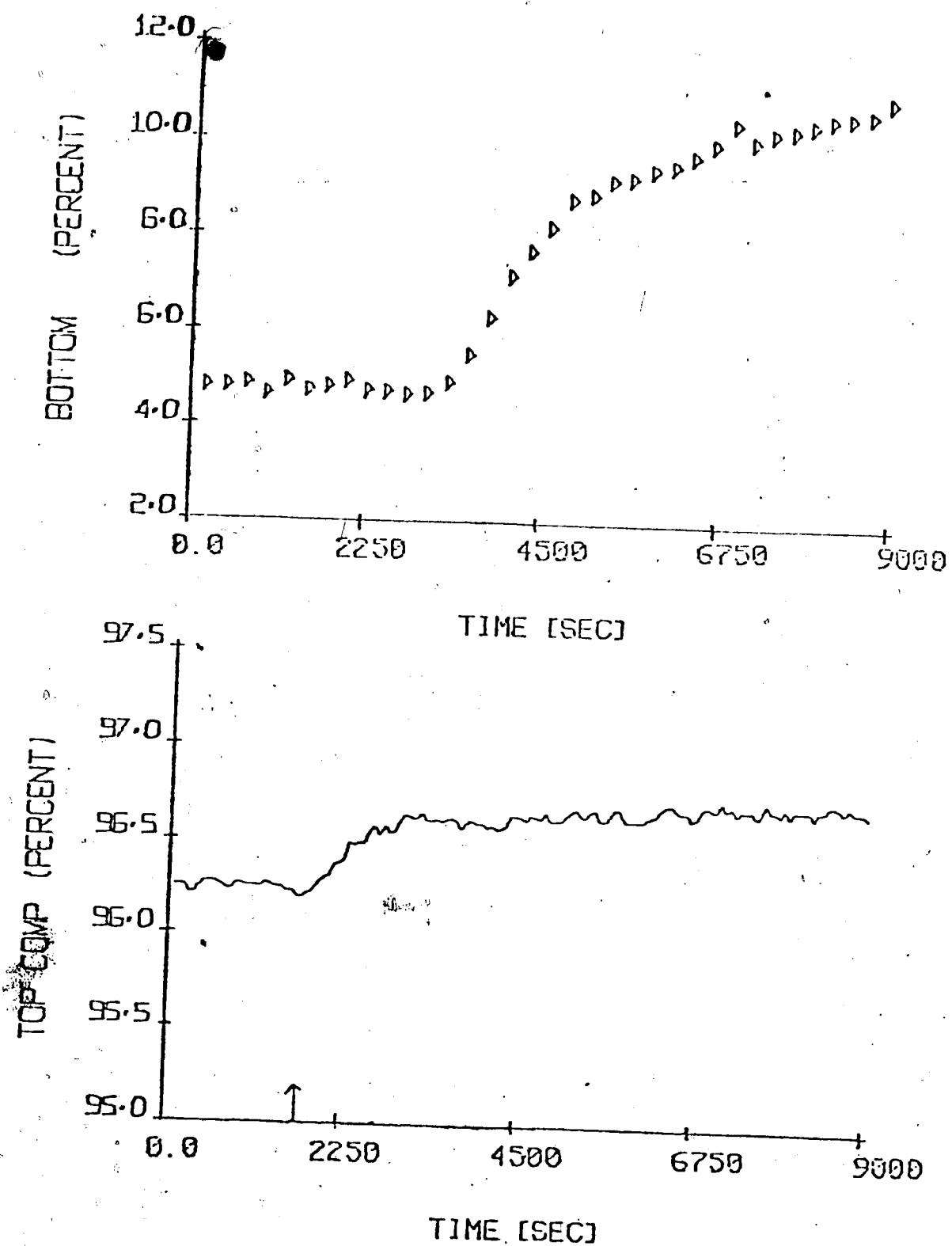
Figure 3.7 Dynamic Response of the Terminal Compositions to a Steam Flow Rate Step Change of -5%
