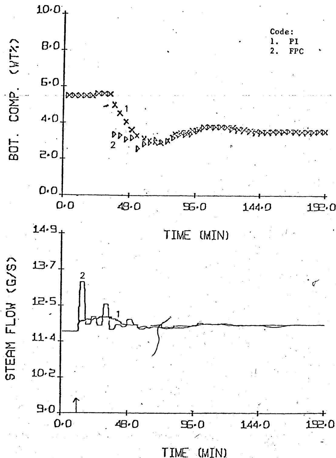
Figure 5.16 Comparison Of Simulation Responses For PI And Multiple Pass FPC Control Of Bottom Product Composition For a 2% Step Decrease In Set Point
