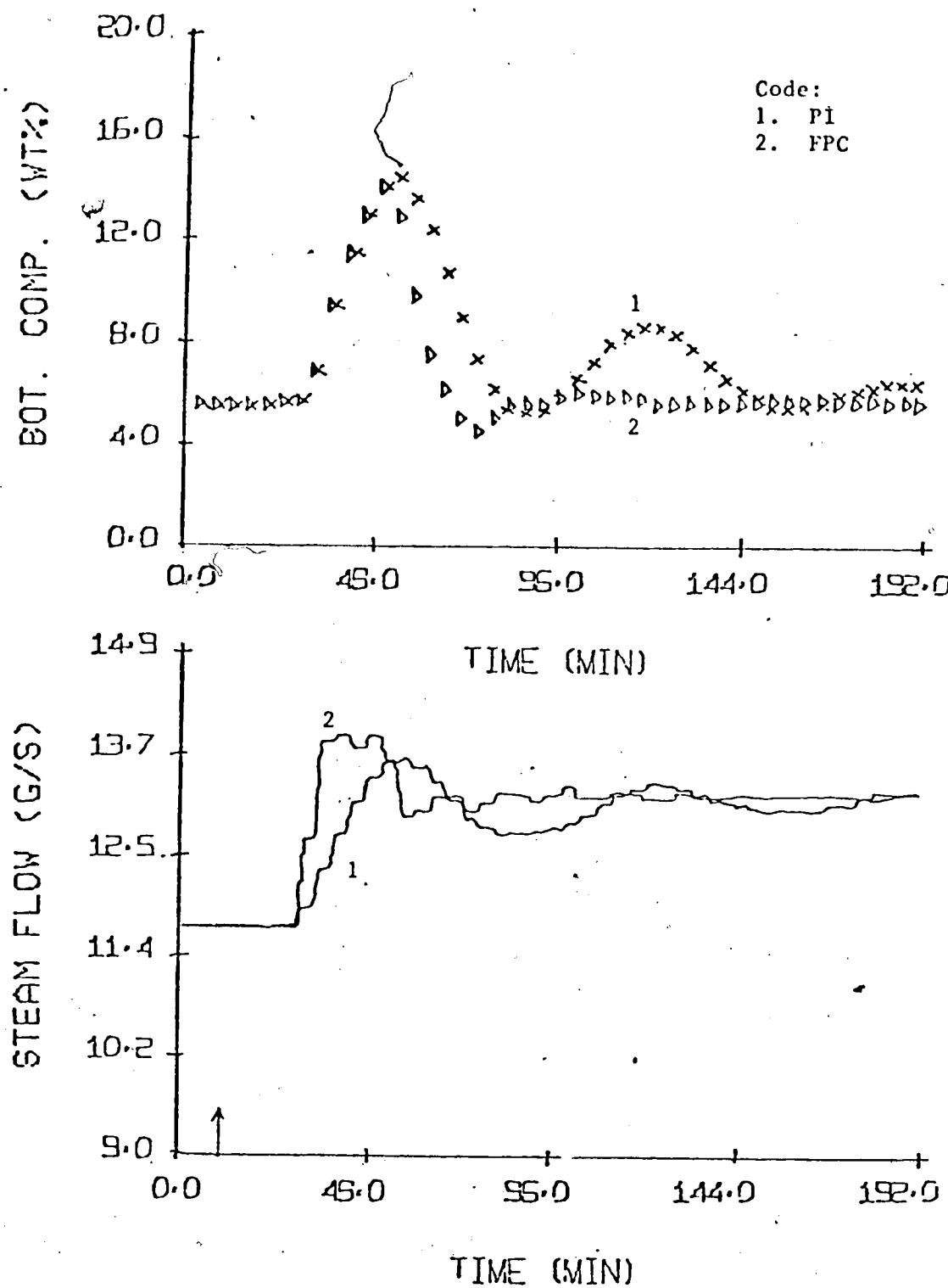
Figure 5.12 Comparison Of Simulation Responses For PI And Multiple Pass FPC Control Of Bottom Composition For a 20% Step Increase In Feed Flow Rate
