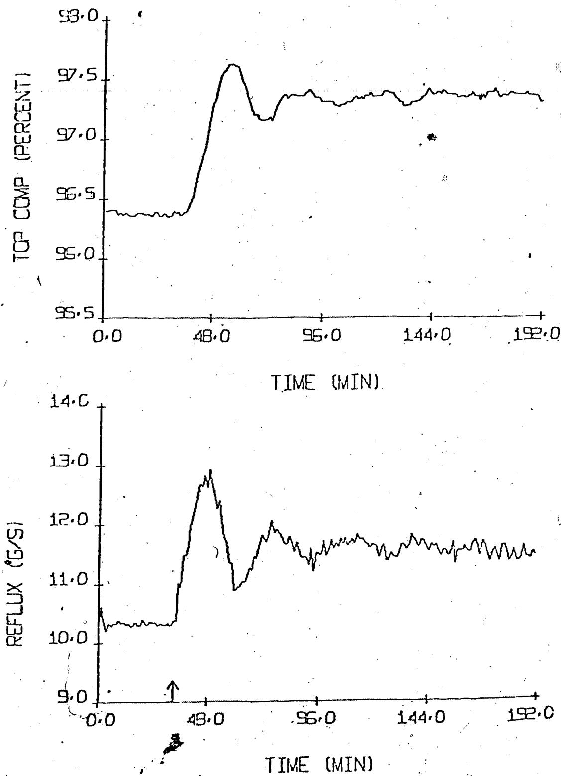
Figure 4.9 Experimental STR Control Of Top Product Composition For a +1% Step Change In Set Point.
