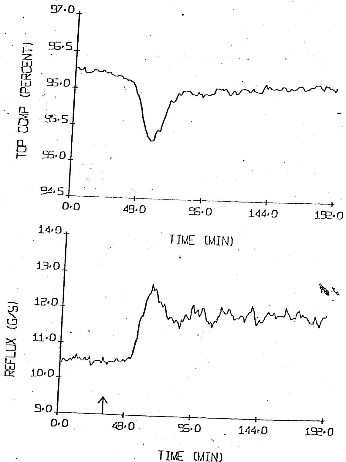
Figure 4.7 Experimental STR Control Of Top Product Composition For a -20% Step Change In Feed Flow Rate:  $\beta_0 = 0.01$ ,  $P(0) = 250$  I.
