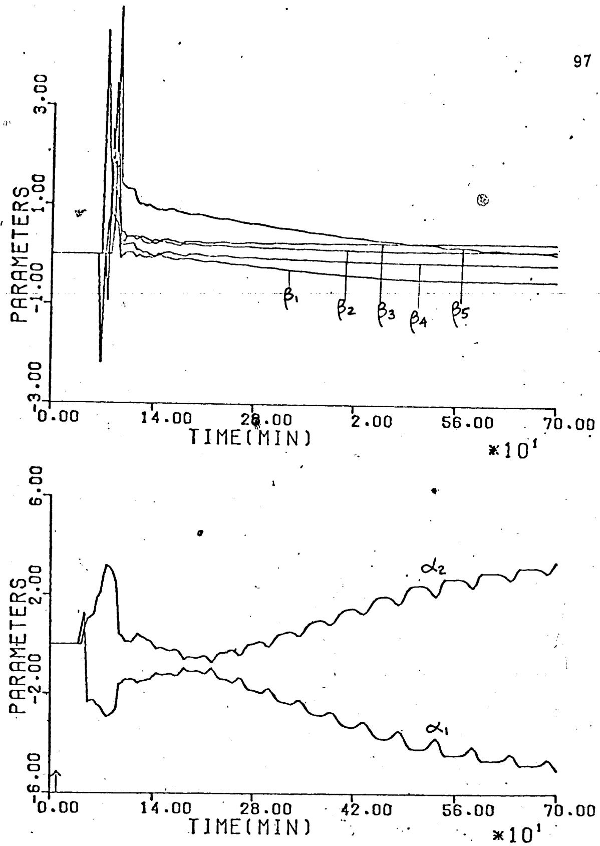
Figure 5.6 Parameter Behavior For Simulated STR Bottom Product Composition Control For a -20% Step Change In Feed Flow Rate, Starting With Zero Initial Parameter Estimates
