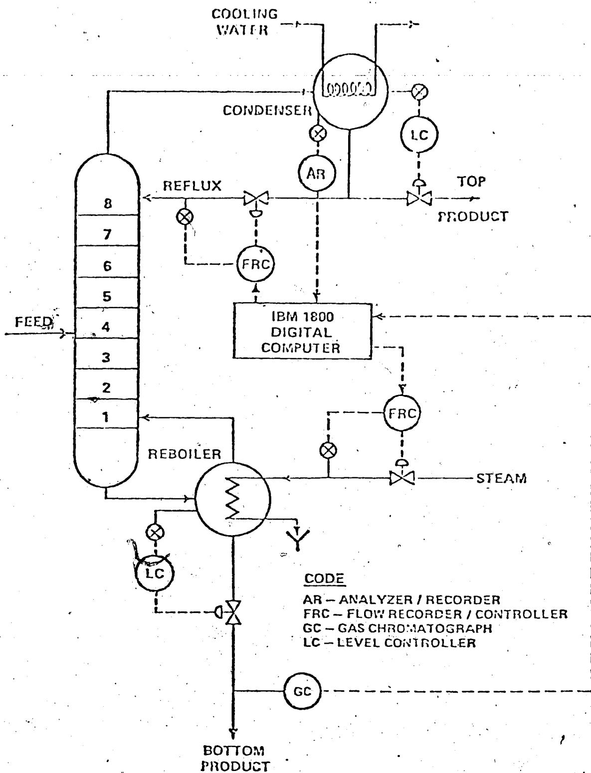
Figure 3.1 Schematic Diagram of the Distillation Column
