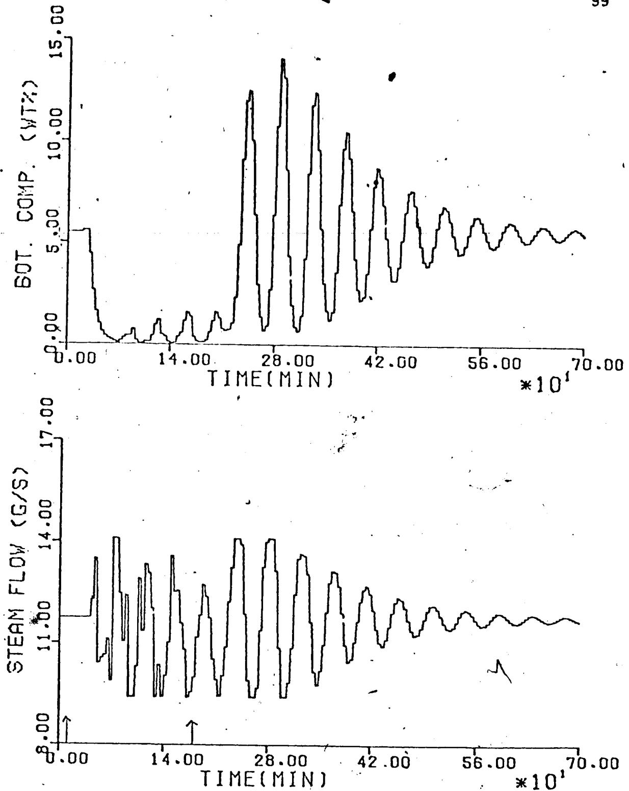
**Figure 5.7** Simulated Response For STR Bottom Product Composition Control For a Pulse Disturbance In Feed Flow Rate Of -3.6 g/s In Magnitude For a Duration Of 170 Minutes, Starting With Zero Initial Parameter Estimates
