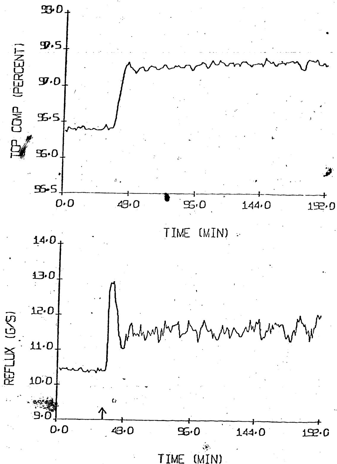
Figure 4.10. Experimental STR Control Of Top Product Composition For a +1% Step Change In Set Point.
