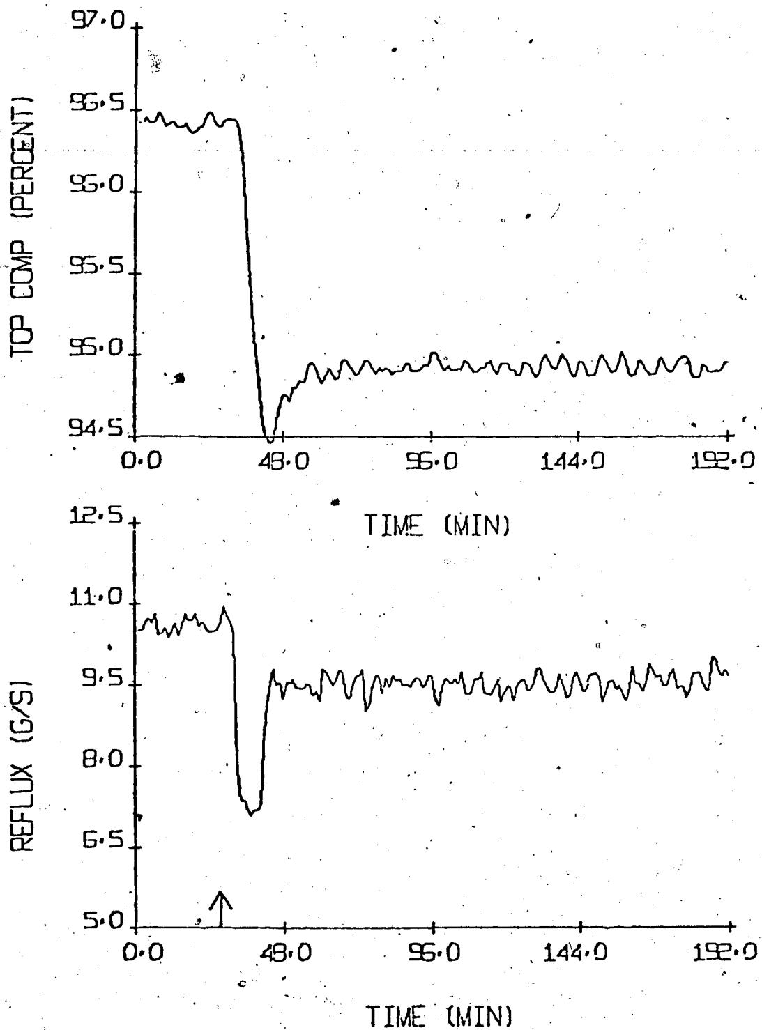
Figure 4.5 Experimental PI Control Of Top Product Composition For a -1.5% Step Change In Set Point
