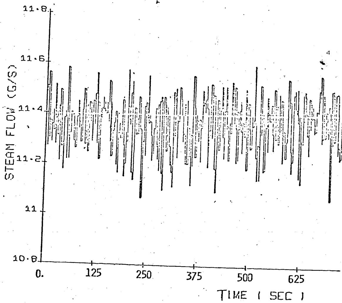
Figure 3.12 Experimental Steady State Steam Flow Noise Display
