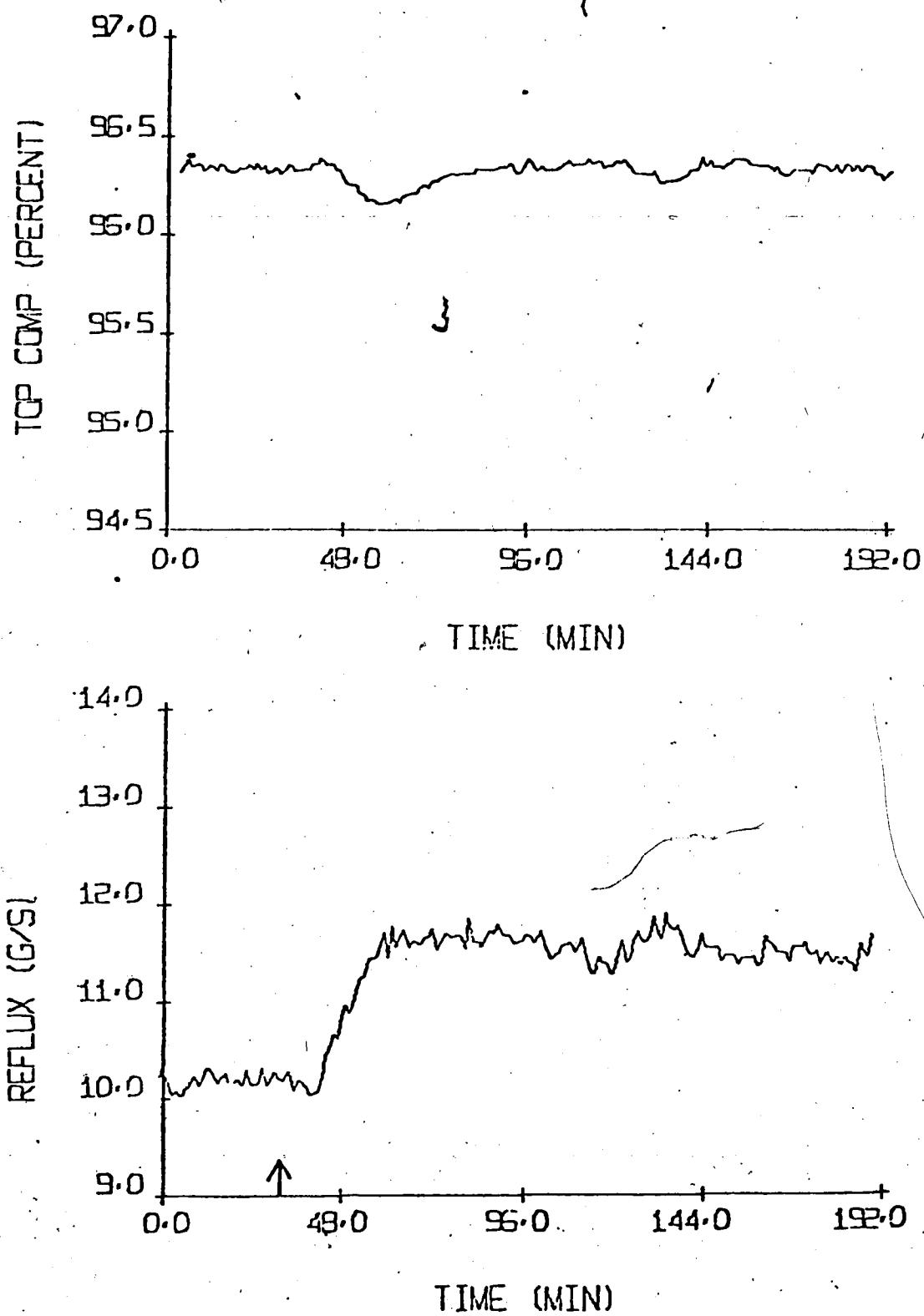
Figure 4.3 Experimental PI Control Of Top Product Composition For a -20% Step Change In Feed Flow Rate
