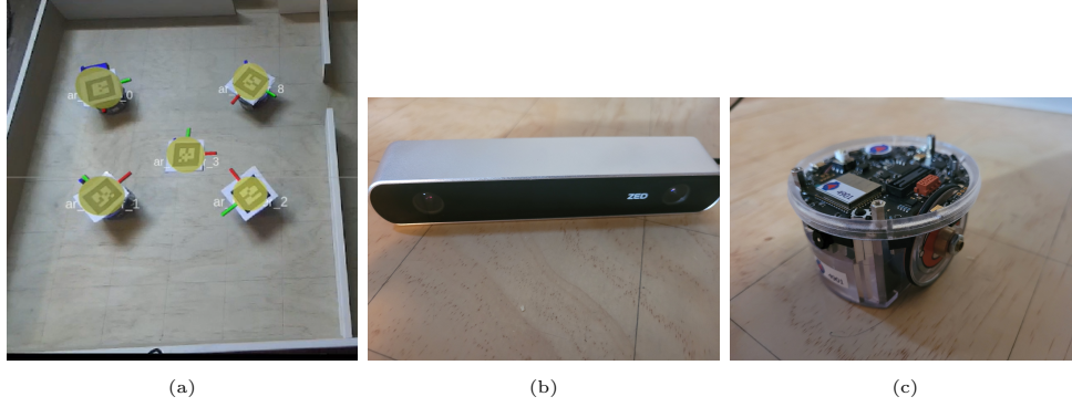
Figure 7.7: Experimental setup including (a) four e-puck2 robots equipped with ArUco tags, (b) overhead ZED camera, (c) e-puck2 robot
