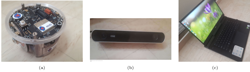
Figure 5.8: Experimental setup including (a) e-puck2 robot, (b) overhead ZED camera, (c) gaming laptop (equipped with Nvidia GPU)
