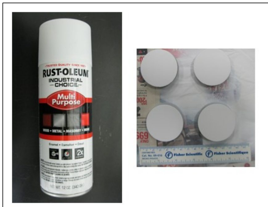
Figure 5.6 Flat white paint used for sample preparation
