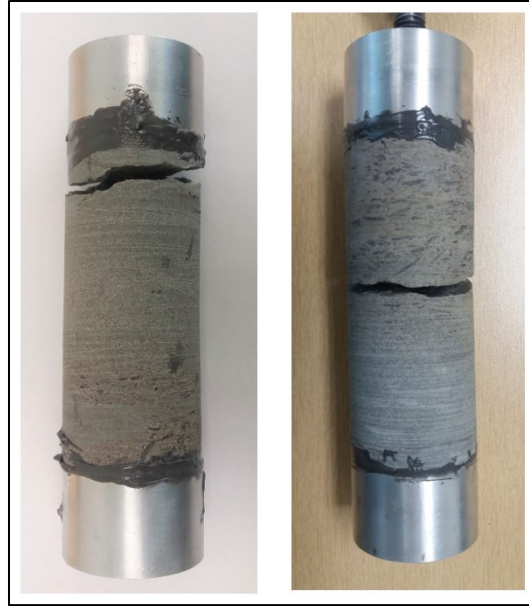
Figure 5.19 The two characteristic crack locations in rock samples after Pull test
