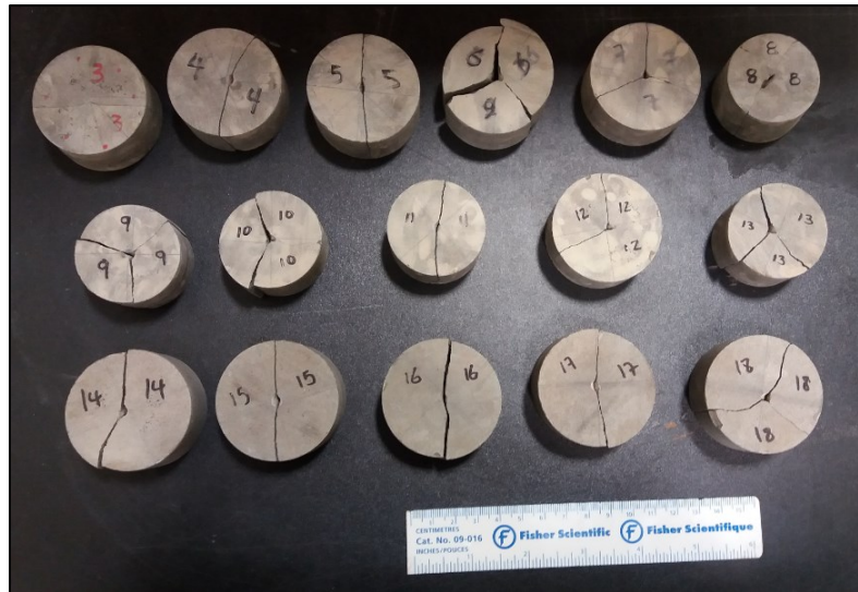
Figure 3.7 Part broken samples under Point Load Test (PLT)
