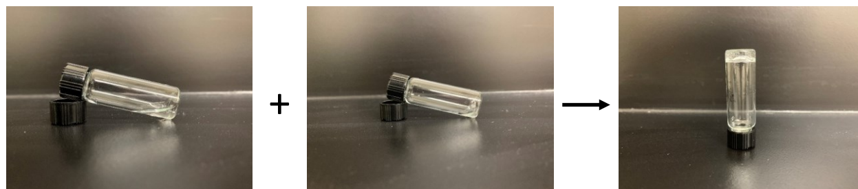
Figure S4.5. After mixing PBS solutions of DPB-PEG4k and P(AM-co-LAEMA), the BL4k hydrogel (boronic acid/sugar=1:1, 10 w/v%) was formed and stayed still when the vial was inverted.
