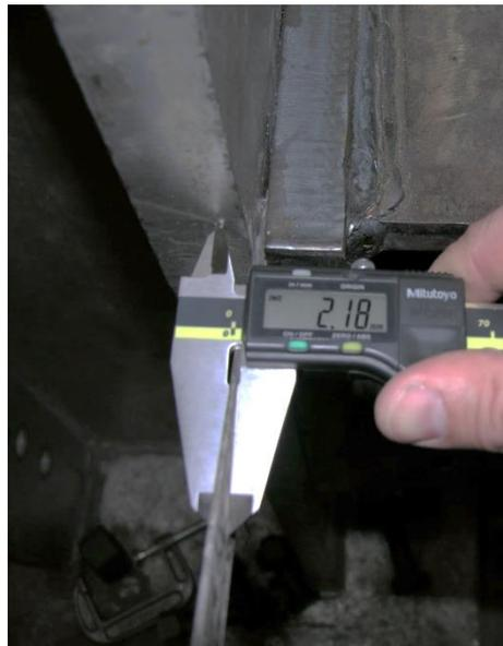
**Figure 4.22. Post-test gap between end plate and strong column (SP9)**
