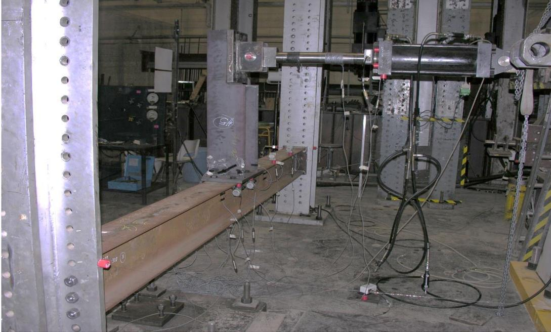
**Figure 4.11. Test specimen in place with instrumentation before the test**
