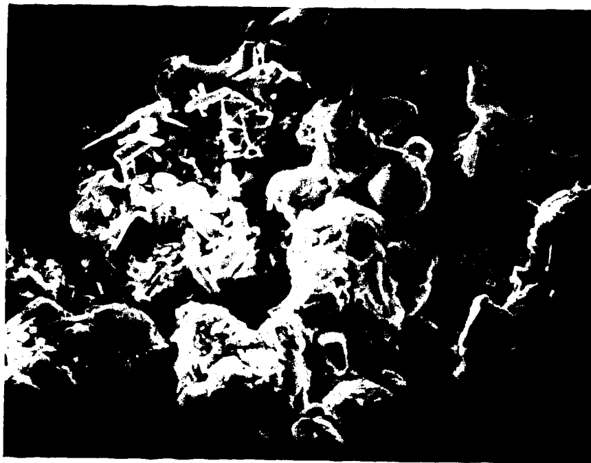
Photograph 6: Luncoor ash after water leaching (100 \mu\text{m} )
