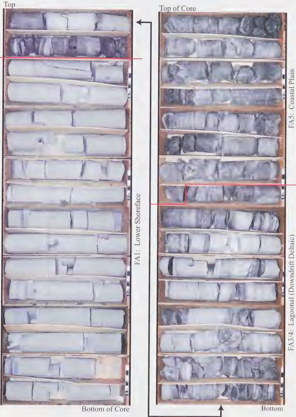
Fig. 3.16 - Deltaic influenced succession located on the downdrift portion of a wave-dominated delta from the Falher D member. The lower half of the core represents a shoaling upward succession deposited within the lower shoreface. These deposits are sharply overlain by lagoonal deposits interpreted to be present in-between barrier bars within the downdrift flank of the delta. Core photos taken from well 15-21-68-08W6, depth 2043.1-2061.6m.
