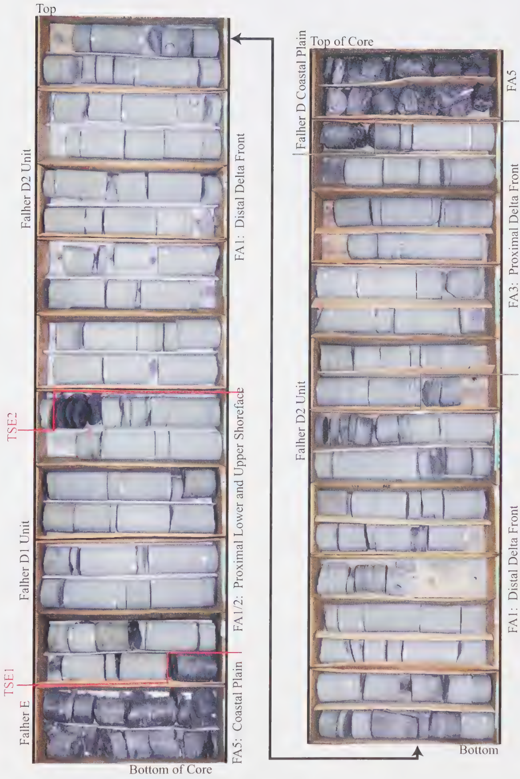
Fig. 4.3 - Deltaic succession from the Falher D member containing both the D1 and D2 intervals. The D2 unit contains a coarsening-upward succession from distal delta front to proximal delta front. The D1 interval contains proximal lower shoreface and upper shoreface deposits. Underlying interbedded coals and mudstones are from the Falher E member. Core photos taken from well located at 10-31-68-10W6, depth 2153.6-2175.7m.
