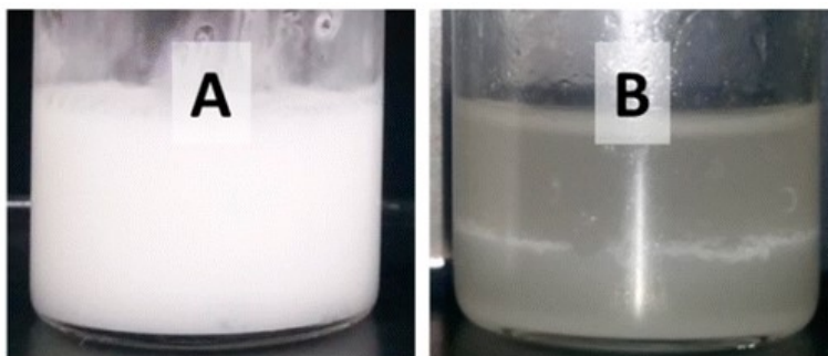
Figure 5-9. Change in interfacial properties of composite absorbent particles after water-absorption. (A) Water-in-mineral oil emulsion stabilized by 2.5 wt% CMC-EC composite particles with initial contact angle of approximately 89^\circ (before absorbing water) and (B) phase separation of the emulsion after 24 h as the particles absorb water and become increasingly hydrophilic with contact angle of approximately 52^\circ .
