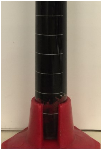
Figure 2-26. High viscosity persistent rag layer formed inside separator. Rag layer accumulates and must be removed by an operator eventually leading to additional process downtime.
