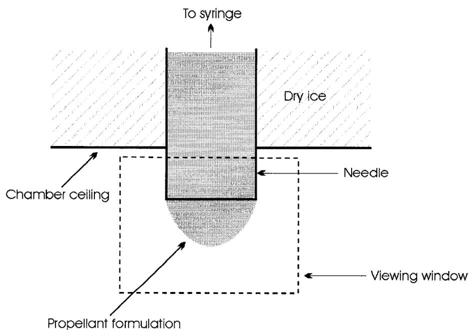
**Figure 3.2** Schematic of droplet suspension into the viewing chamber.
