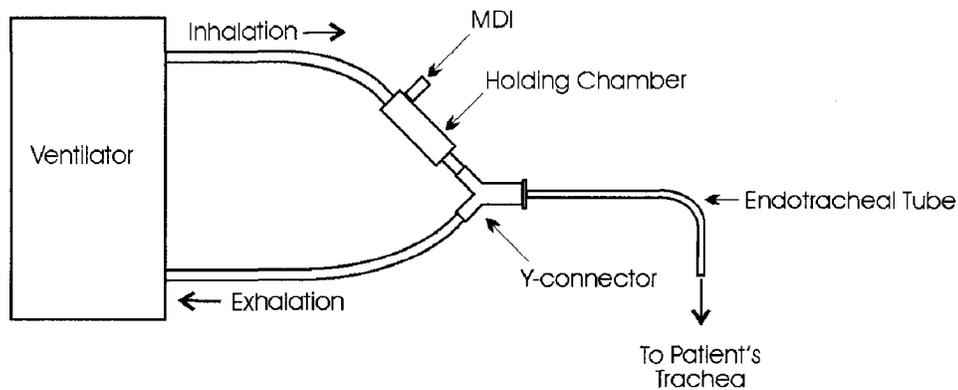
**Figure 1.3** Schematic of ventilator circuit with in-line holding chamber for MDI delivery.
