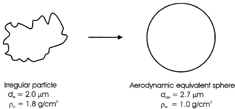
**Figure 2.1** An irregular particle with density of  $1.8 \text{ g/cm}^3$  and volume equivalent to that of a sphere with diameter of  $2.0 \mu\text{m}$  is converted to its aerodynamic equivalent sphere.
