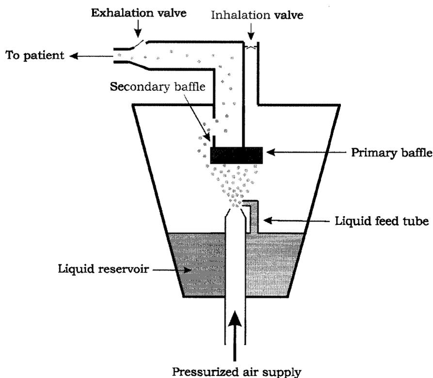
**Figure 1.1** Schematic of a typical nebulizer design (adapted from Finlay (4)).
