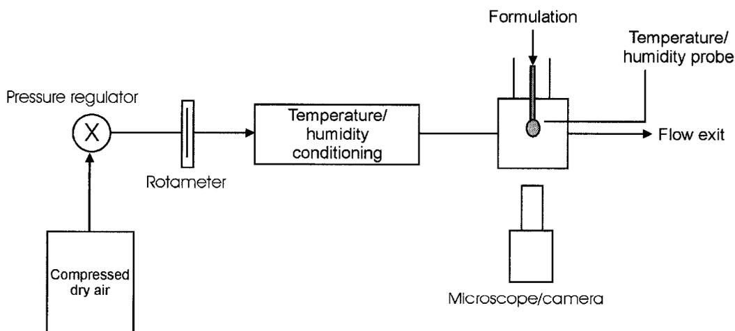
**Figure 3.1** Schematic of the experimental apparatus for pendant droplet experiments.
