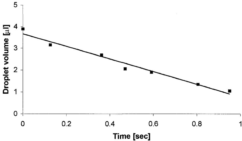
**Figure 4.1** Volume versus time data for an evaporating droplet of pure HFA 227ea propellant at 37° C and <10% RH. Line represents a linear least-squares fit of slope  $-2.9\mu\text{l}/\text{sec}$  ( $R^2 = 0.9729$ ).
