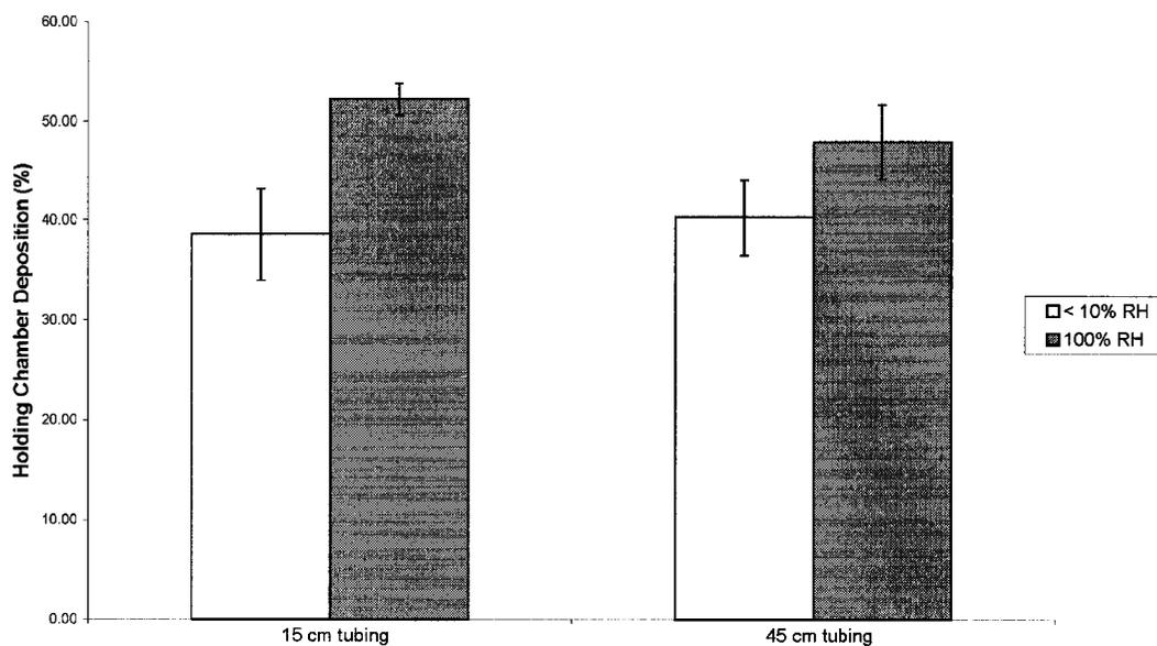
**Figure 4.3** The percentage of drug depositing in the holding chamber from the AiroMir® MDI in dry compared to humid airflow. Results are shown for experiments with two different lengths of tubing separating the holding chamber from the cascade impactor. Error bars represent one standard deviation.
