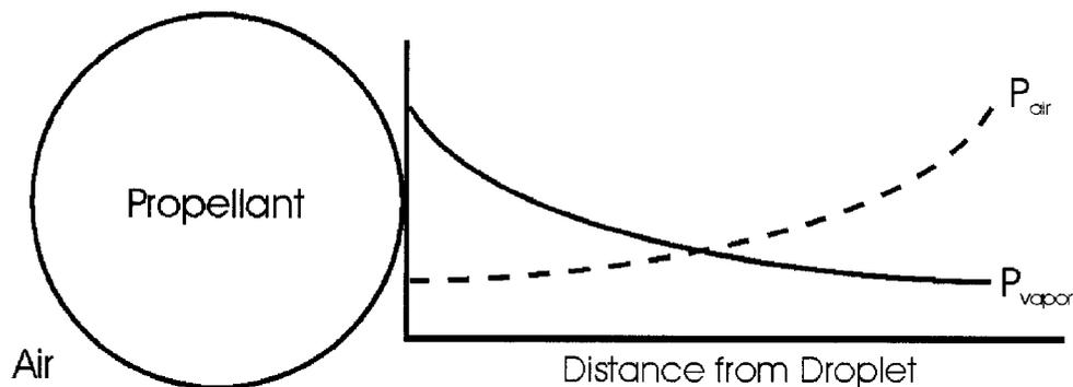
**Figure 2.5** Pressure gradients in an air/vapor mixture with distance from the droplet surface.
