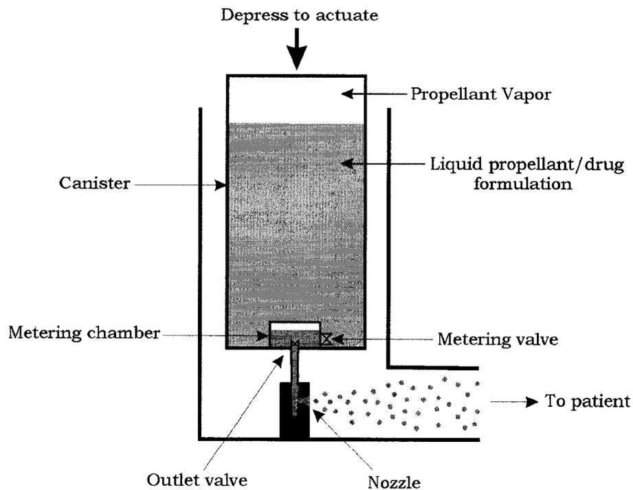
**Figure 1.2** Schematic of a typical MDI design (adapted from Finlay (4)).
