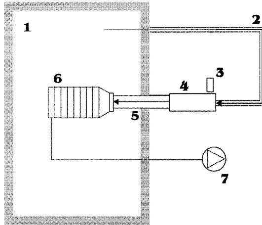
**Figure 3.6** Schematic diagram of the bench test: 1 climatized chamber; 2 insulated inspiratory tubing; 3 MDI canister; 4 holding chamber; 5 tygon tubing; 6 cascade impactor; 7 vacuum pump (28.3 l/min).
