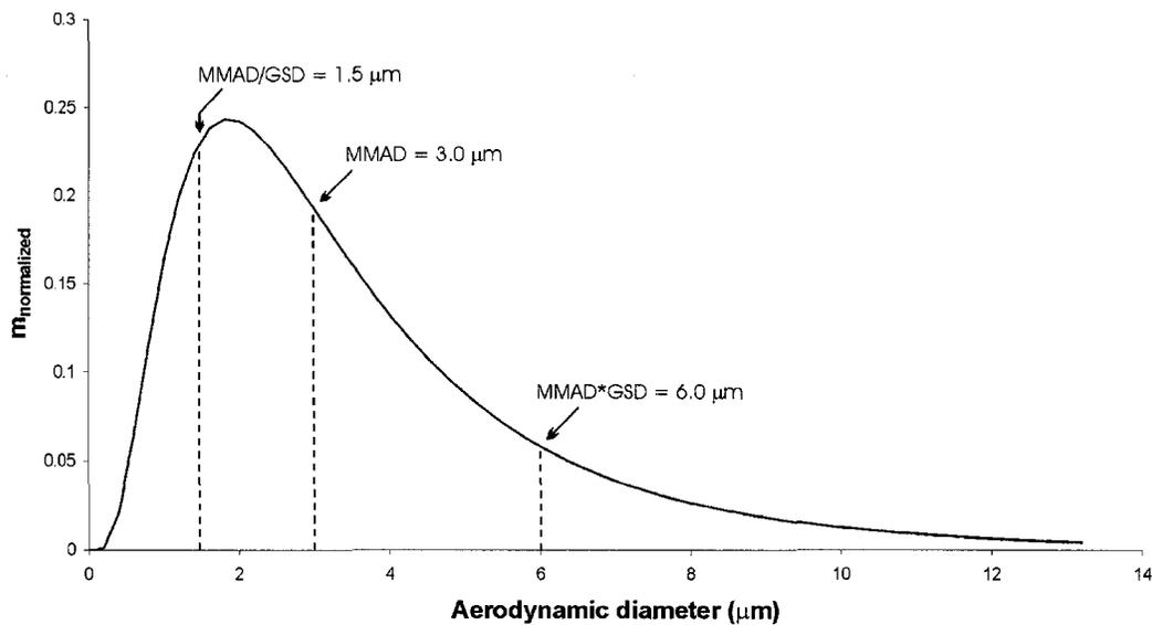
**Figure 2.2** Normalized log-normal mass distribution with MMAD = 3.0  $\mu\text{m}$  and GSD = 2.0. 68% of the total aerosol mass is contained in particle sizes between MMAD/GSD and MMAD\*GSD.
