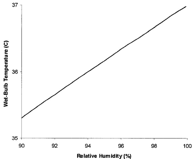
**Figure 5.1** Wet-bulb temperatures for water droplets in 37° C air.
