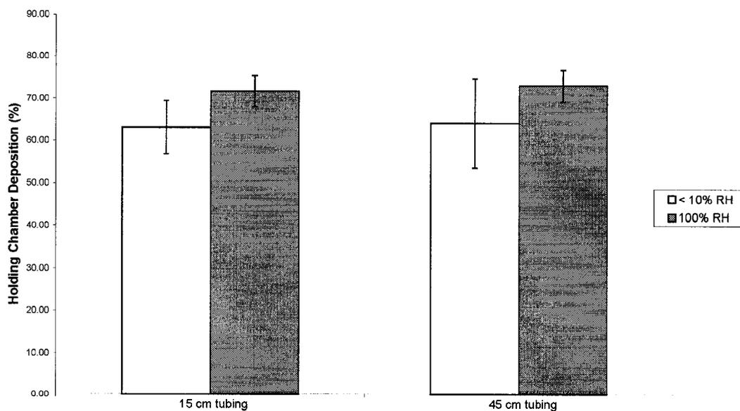
**Figure 4.4** The percentage of drug depositing in the holding chamber from the Ventolin® HFA MDI in dry compared to humid airflow. Results are shown for experiments with two different lengths of tubing separating the holding chamber from the cascade impactor. Error bars represent one standard deviation.
