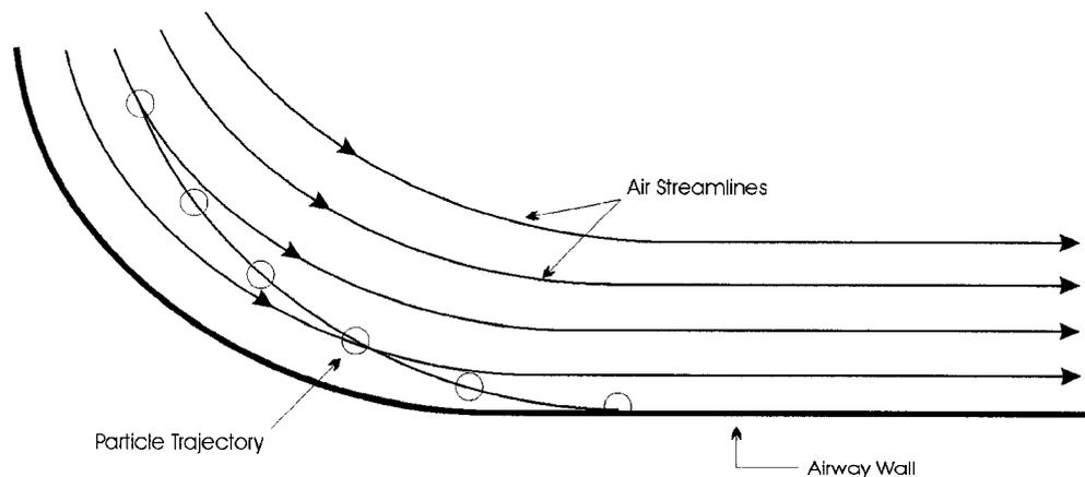
**Figure 2.4** Particle deposition by inertial impaction.
