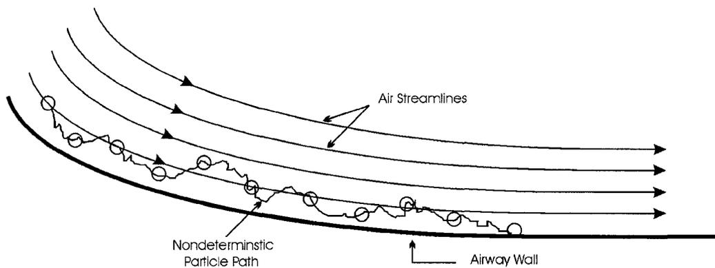
**Figure 2.3** Particle deposition by Brownian diffusion.
