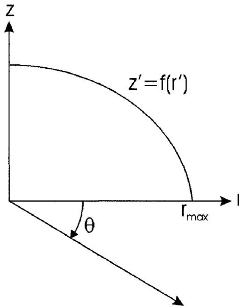
**Figure 3.5** The droplet profile is rotated 180° and a cylindrical coordinate system is introduced in order to determine droplet volume by integration.  $z'$  and  $r'$  are arrays holding the profile coordinates in the  $z$  and  $r$  directions.
