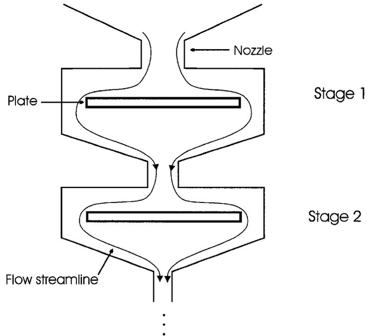
**Figure 3.7** Schematic of the first two stages of a cascade impactor.
