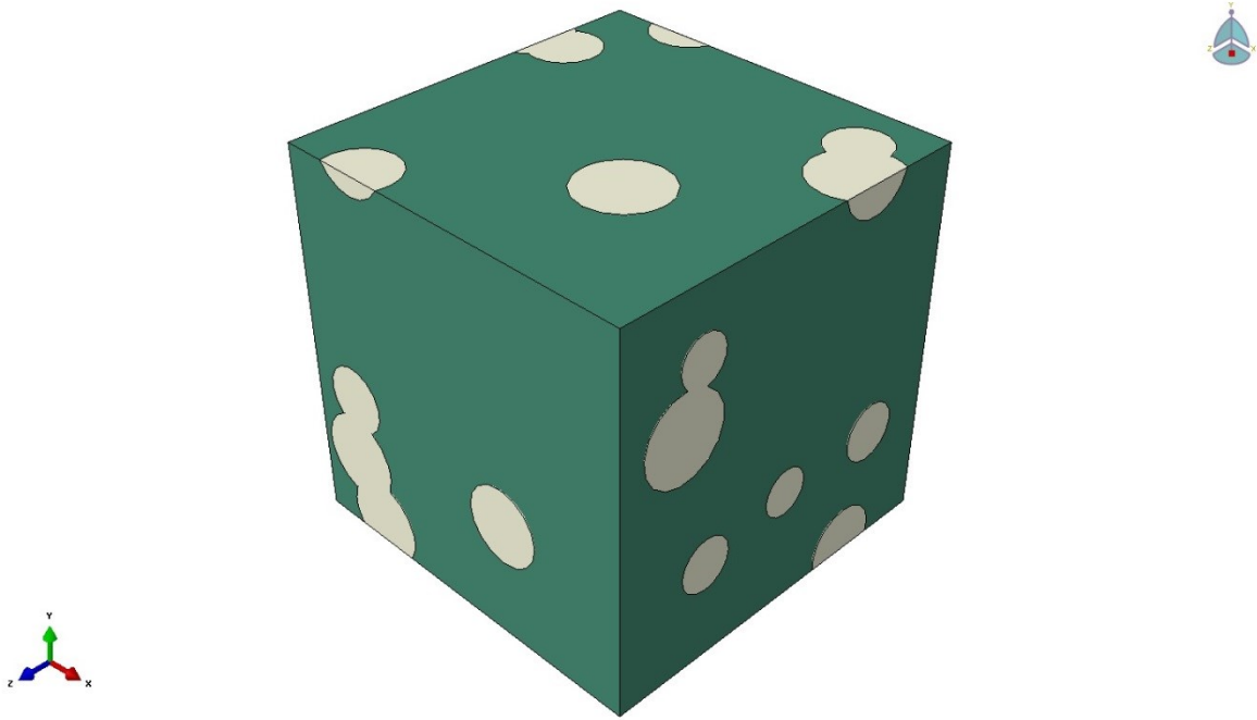
(b) Micromechanical model with 15% volume fraction of particles
