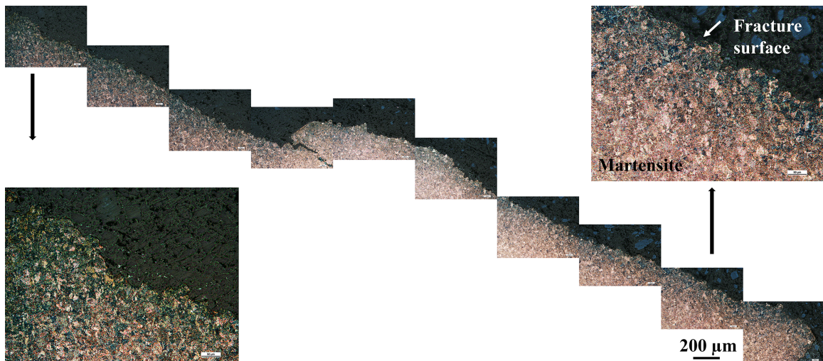
Figure 3.13: Montage of microstructure at the cross section of the fracture surface.
