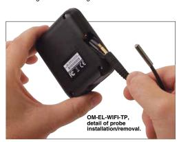
The OM-EL-WIFI Series are low powered battery devices. When configured using typical sampling periods (e.g. once every 5 minutes) the data logger will operate for over one year. The battery can then be recharged via a PC or USB 5V wall adaptor using the USB lead provided
