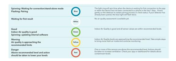
For details on sensor thresholds go to airthings.com/wave-plus
