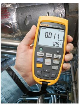
Today's HVAC technicians need a simple solution for diagnosing ventilation issues. The Fluke 922 makes airflow measurements easy by combining pressure, air flow, and velocity into a single, rugged meter. Compatible with most pitot tubes, the Fluke 922 allows technicians to conveniently enter their duct shape and dimensions for maximum measurement accuracy.
