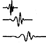
Figure 4.2: Dilation of a function
