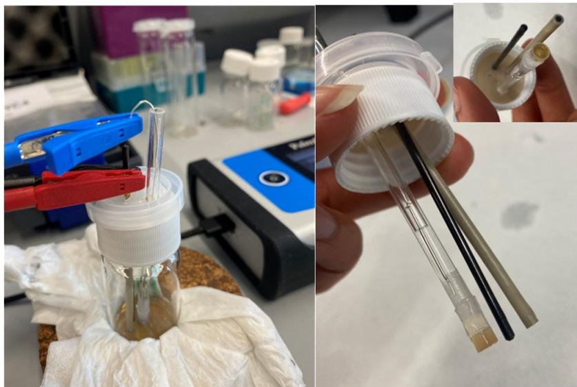
**Figure 3-A4.** Electrode set-up derived for use with the PalmSens4 potentiostat. Showing the lead attachment (left) and the appearance of the Ag/AgCl reference, graphite counter, and graphite working electrodes (right).
