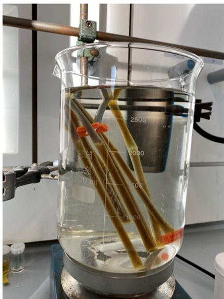
**Figure 3-A2.** Dialysis setup used for purification of the CNDs and CND@AQCA.
