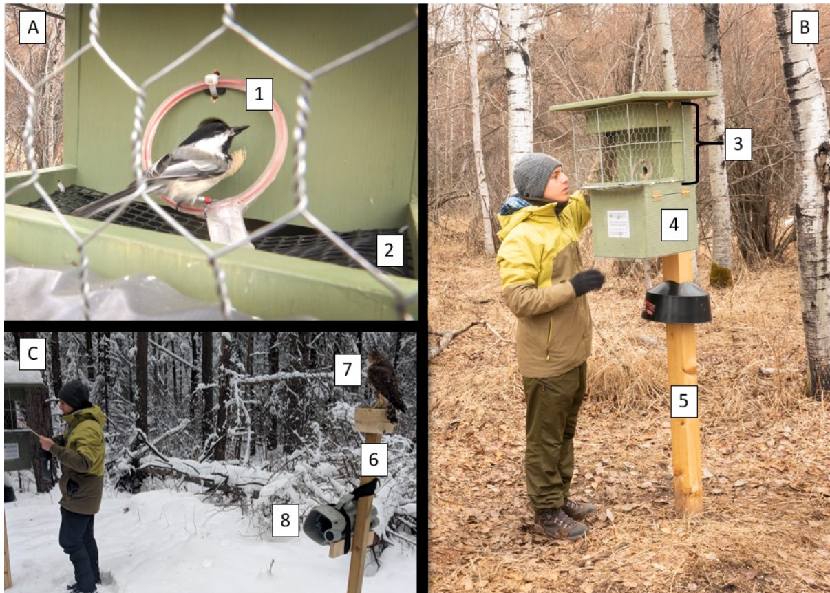
Figure S3. Feeder set up and detailed information of the feeder. A: Close up of a chickadee taking a seed out of the feeder. 1: RFID antenna reader. 2: Fine mesh to prevent feeding from the ground. B: Overall visualization of the feeder setup. JAT next to the feeder. 3: Wire mesh to protect the feeder and prevent small mammals and other birds from accessing the seeds. 4: Side access door to the battery and RFID readers. 5: Base pole of the feeder. All feeders were installed at the same height with the seed hole at approximately 1.60 m. C: Example of a acoustic+visual treatment and overview of the set-up. 6: Experimental pole. 7: Merlin mount. 8: Speaker broadcasting chickadee mobbing calls. © A and B: Megan A. Westervelt; C: Jan Wijmenga
