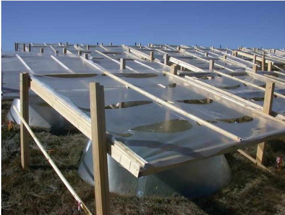
Plate 2-1. Picture showing experimental plots with rain-out shelters. The one directly above has slits to allow rainfall penetration and has an OTC underneath.
