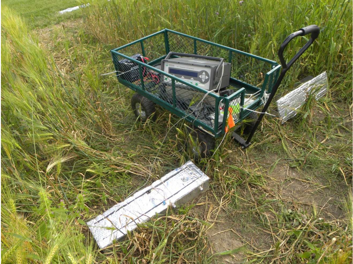
Figure 2.3: Photoacoustic multi gas analyzer connected to the active chamber through tubing
