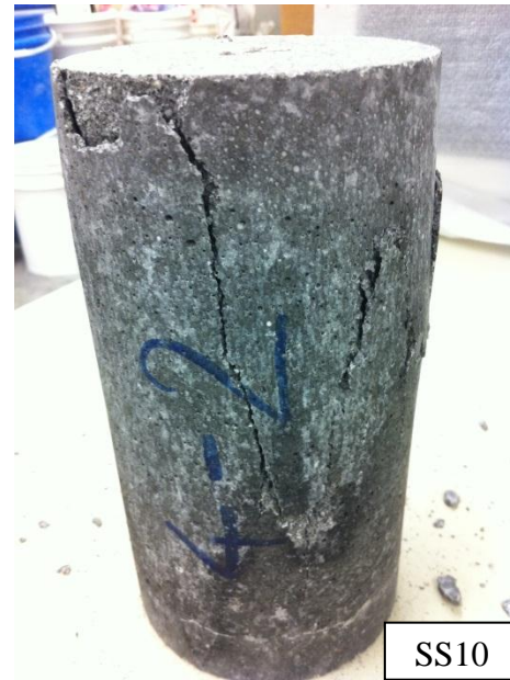
Figure 5-6: Typical failure of cylinder specimens of mixes SS5 and SS10
