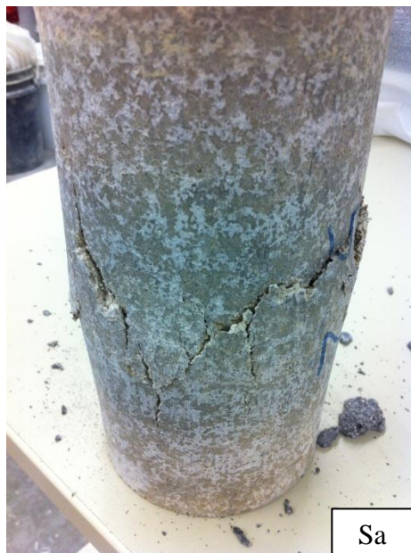
Figure 5-7: Typical failure of cylinder specimens of mixes Sa and SaB
