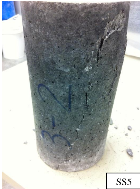
Figure 5-6: Typical failure of cylinder specimens of mixes SS5 and SS10
