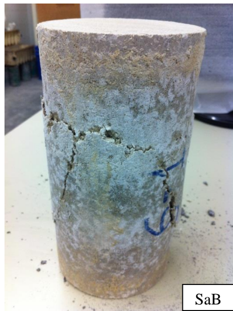
Figure 5-7: Typical failure of cylinder specimens of mixes Sa and SaB
