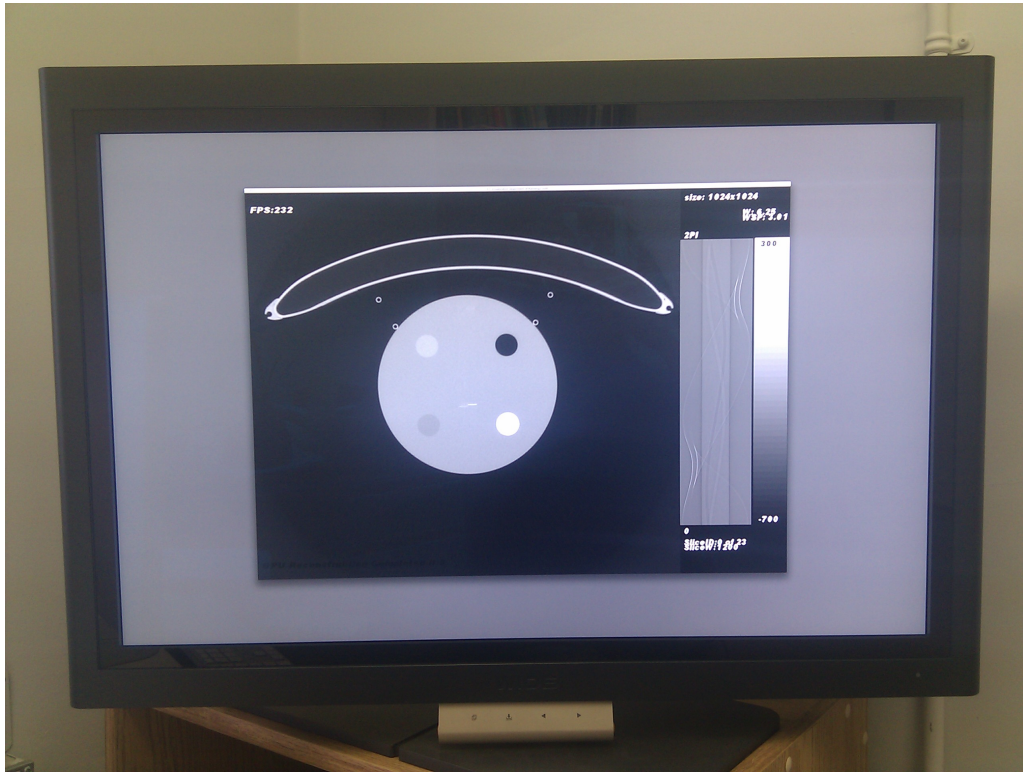
Figure 4.5: AREMI is seen displayed on the 14-bit PAC display in monochrome mode. The ability to output HDR to the monitor is likely beneficial to diagnostic imaging specialists.
