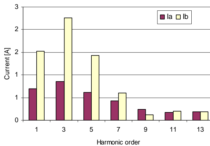
Figure 6-10 Harmonic spectrum of currents measured at the PCC ( I_1 divided by 10).
