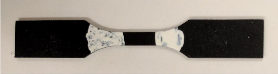
**Figure 2-5: Dog bog sample of Type V dimension of ASTM D638-14 with white paint marking for digital strain measurement**
