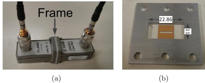
Figure 3.21. (a) Measurement setup including two WR90 waveguides and the frame housing the unit cell; (b) Frame with a unit cell fixed inside.
