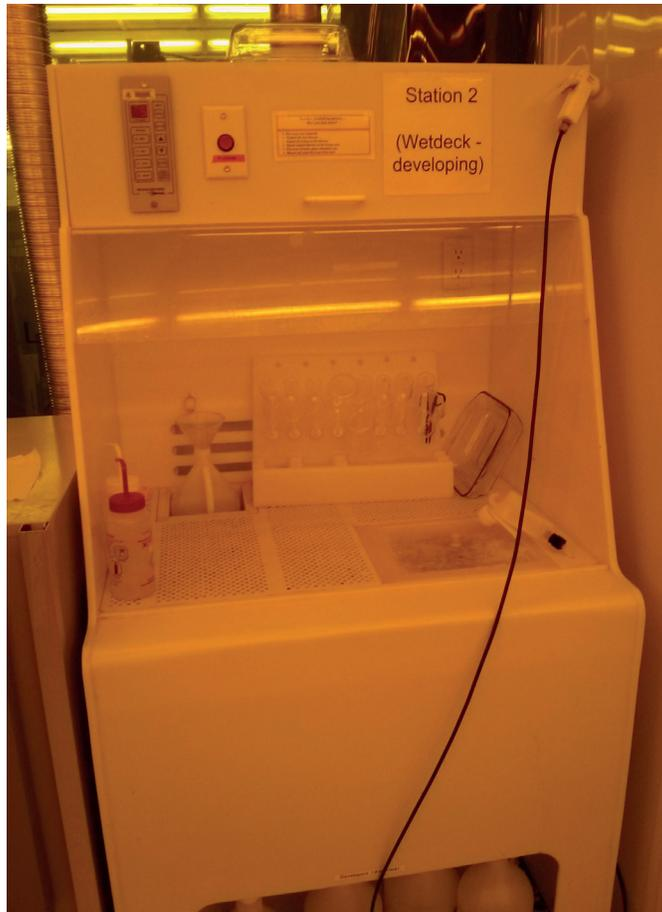
Figure A.5. Wet-deck used for developing the photo-resist.
