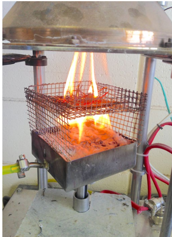
Figure A1. Modified setup for the cone calorimeter flammability testing.
