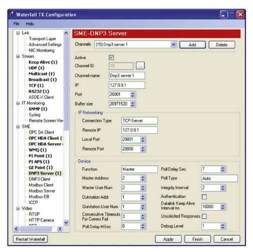
Figure 6 – DNP3 Unidirectional Configuration
