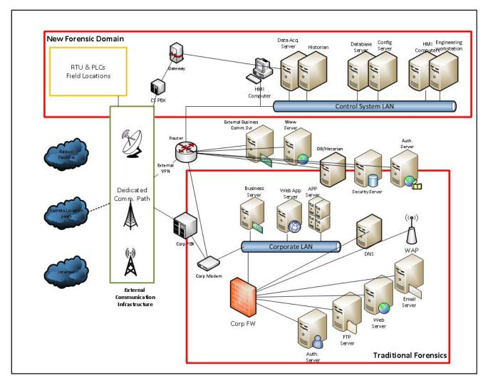
Figure 1 – Control System Physical Architecture
