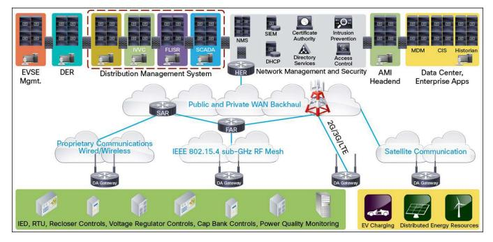
Figure 4 – Field Area Networks (Communication Networks for Smart Grids - Making Smart Grid Real, 2014)
