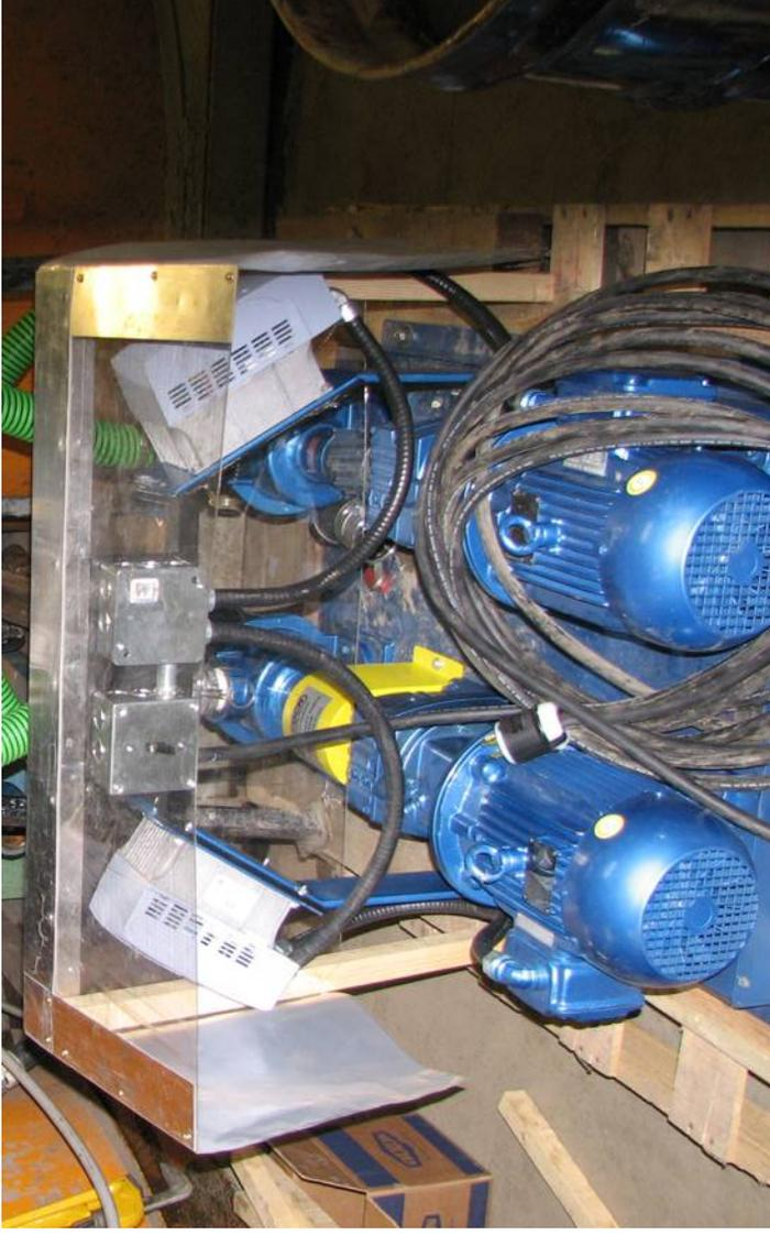
Figure 2.10 Photograph of twin Monyo® 500 36701 progressing cavity pump
