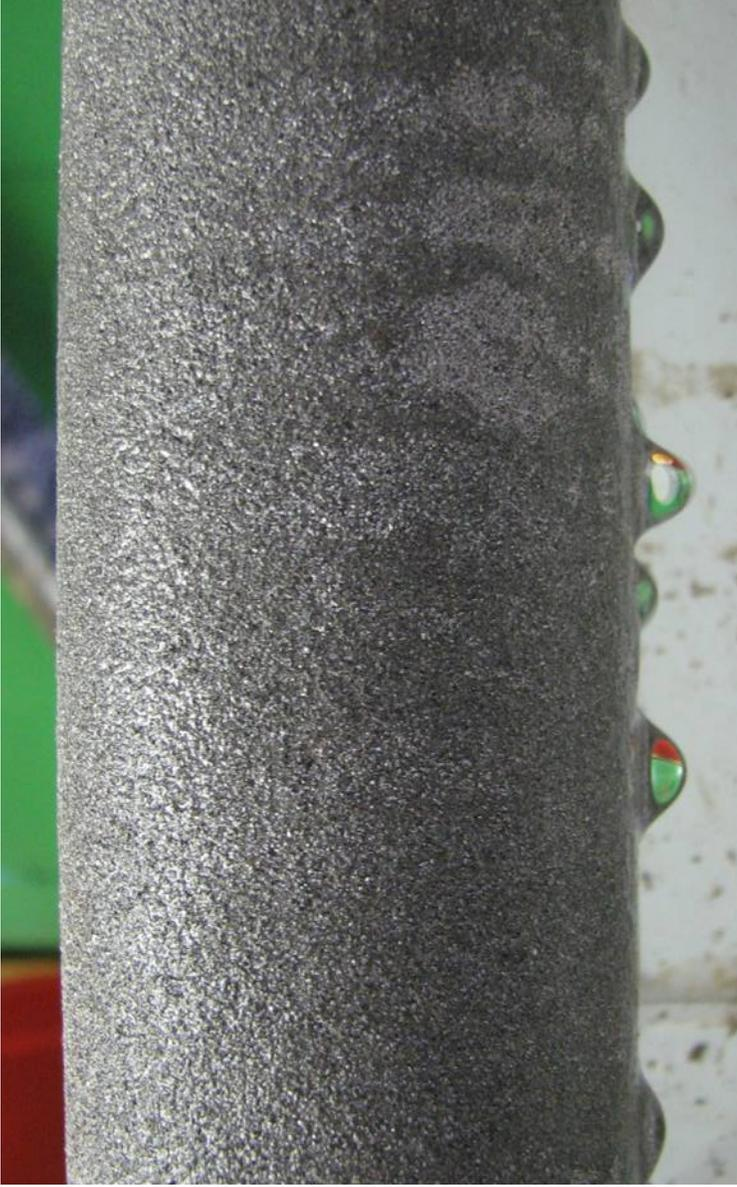
Figure 2.13 Photograph of clean filtrate water drop during test operation
