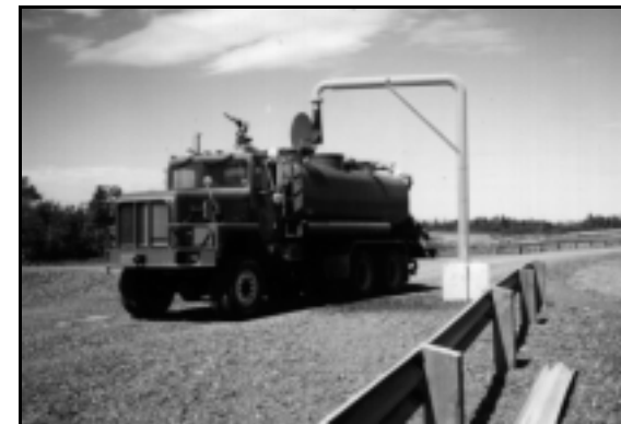
Water Truck Loading from Gantry at Point Aconi Ash Site
