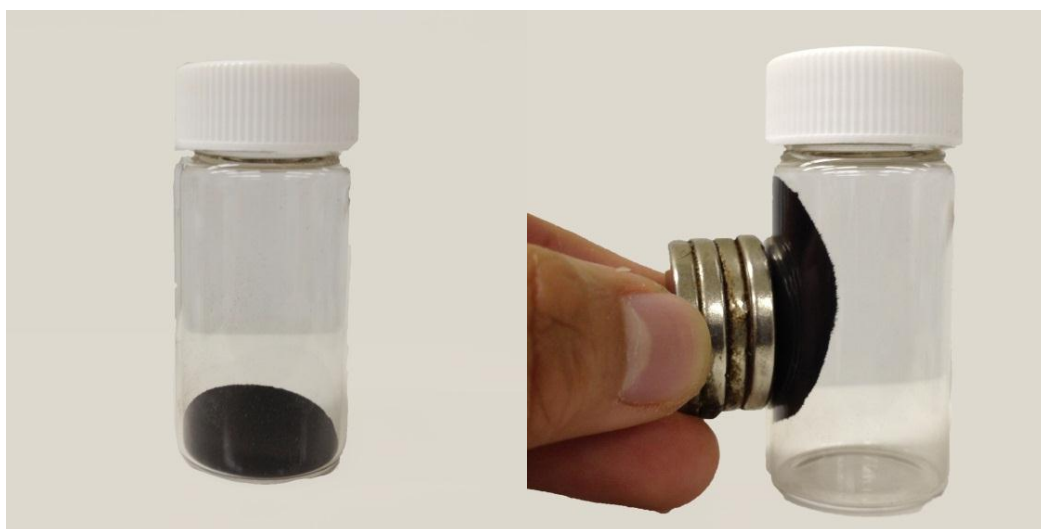
Figure 4.1 M-AC particles attracted by a hand magnet
