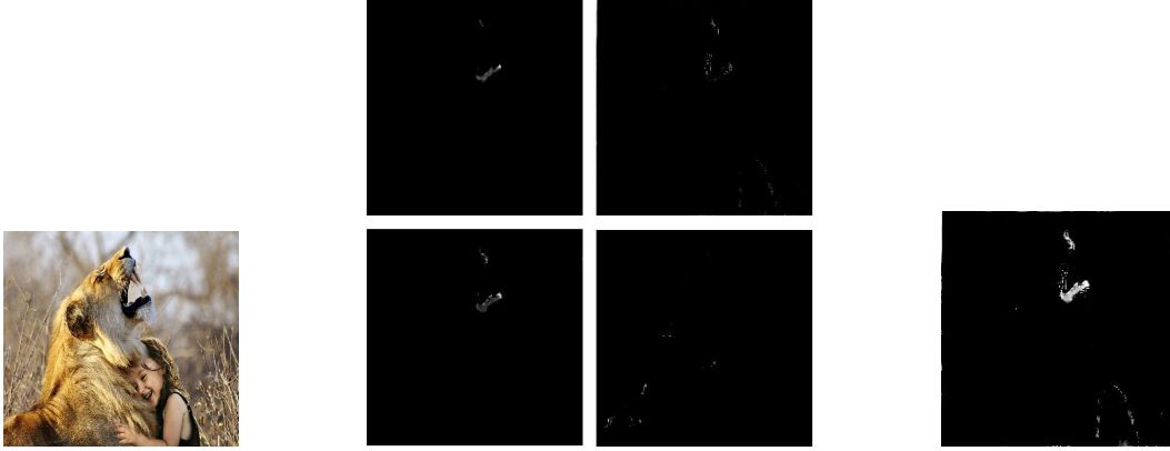
Figure 3.2: Representation of four sample feature maps (middle) of a sample image(left) with their first PC (right).
