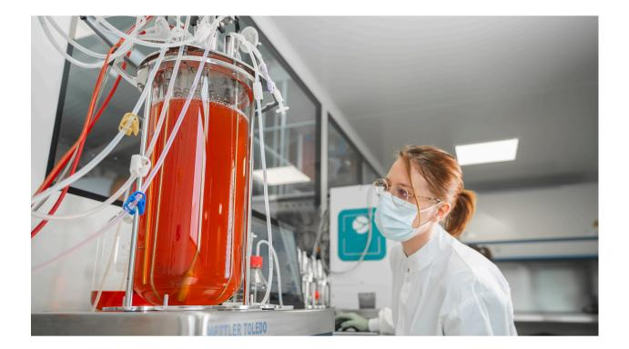
**Figure 2.1.3 Commercial sized bioreactor from TreeFrog therapeutics providing an example of expansion capacity for stem cells within large 3D culture conditions.** Image reproduced with permission from TreeFrog therapeutics <sup>83</sup>.
