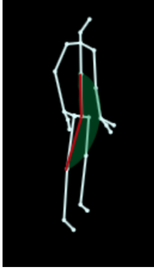
Figure 3.3: The angle between two vectors : spine-base to spine-mid, and spine-base to knee which is used to determine the standing up and sitting down positions ( \alpha_{TUG} ).
