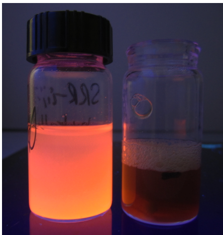
Figure 3.8: Qualitative PL from; Left- Mesoporous silica encapsulated Si-NCs in water, Right- CTAB/Si-NC emulsion 3 hours after base addition
