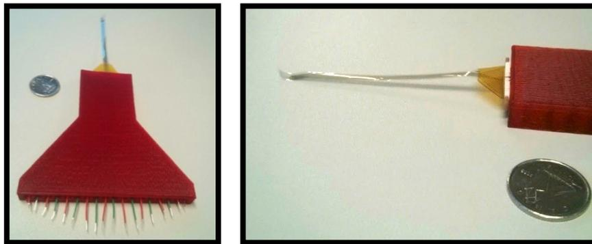
**Figure 32** – Images of a  $\mu$ ECoG Probe mounted into a ZIF-Connector device taken from two different angles (dimes for scale).
