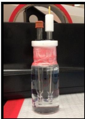
**Figure 68** – A properly stored non-aqueous Ag|Ag<sup>+</sup> RE being kept in a storage container filled to an adequate level with the appropriate storage solution.
