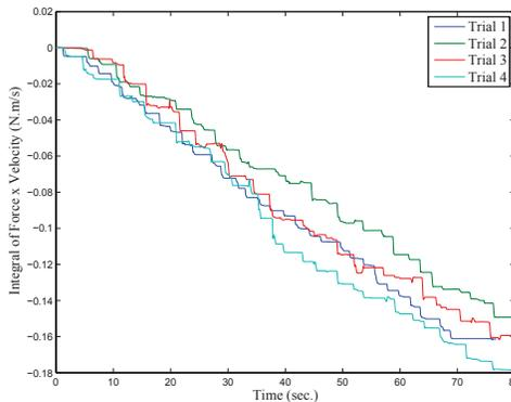
Figure 4: The integral of force times velocity is an indication of passivity. Becoming negative implies that the system is non-passive. The operator is asked to voluntarily apply perturbations to the robot.
