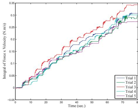
Figure 3: The integral of force times velocity is an indication of passivity. Staying non-negative for all times corresponds to passivity of the system. The operator is asked to have his arm on the robot but does not apply any deliberate force to the robot.
