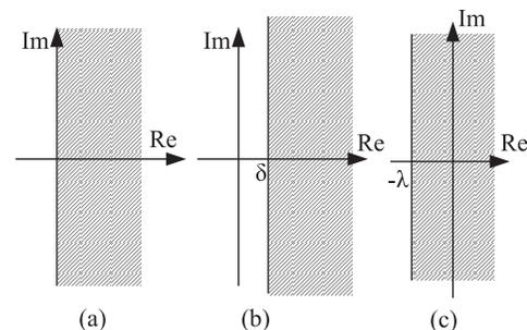
Figure 2: Nyquist diagrams of (a) a passive system, (b) an ISP system with excess of passivity of  $\delta$ , (c) a non-passive system with shortage of passivity of  $\lambda$ .
