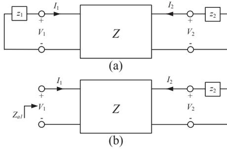
Figure 5: (a) Two-port network and (b) driving-point impedance  $Z_{a1} = V_1/I_1$  when port 2 is terminated to a passive impedance  $z_2$ .
