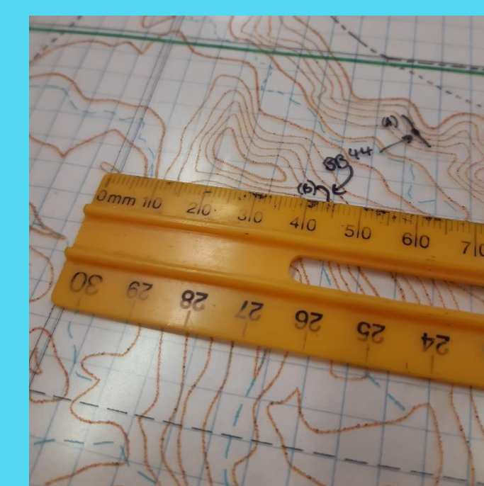
Figure 4: A ruler being used to find a point's coordinates. 1 mm on the map represents 10 m in the park.
