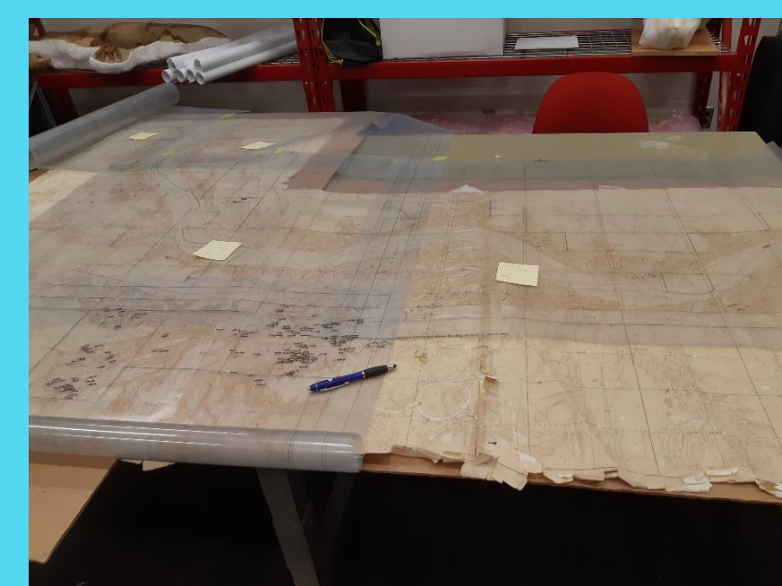
Figure 3: Mylar maps overlaying a paper map. The mylar maps were carefully matched to the paper maps and taped in place.
