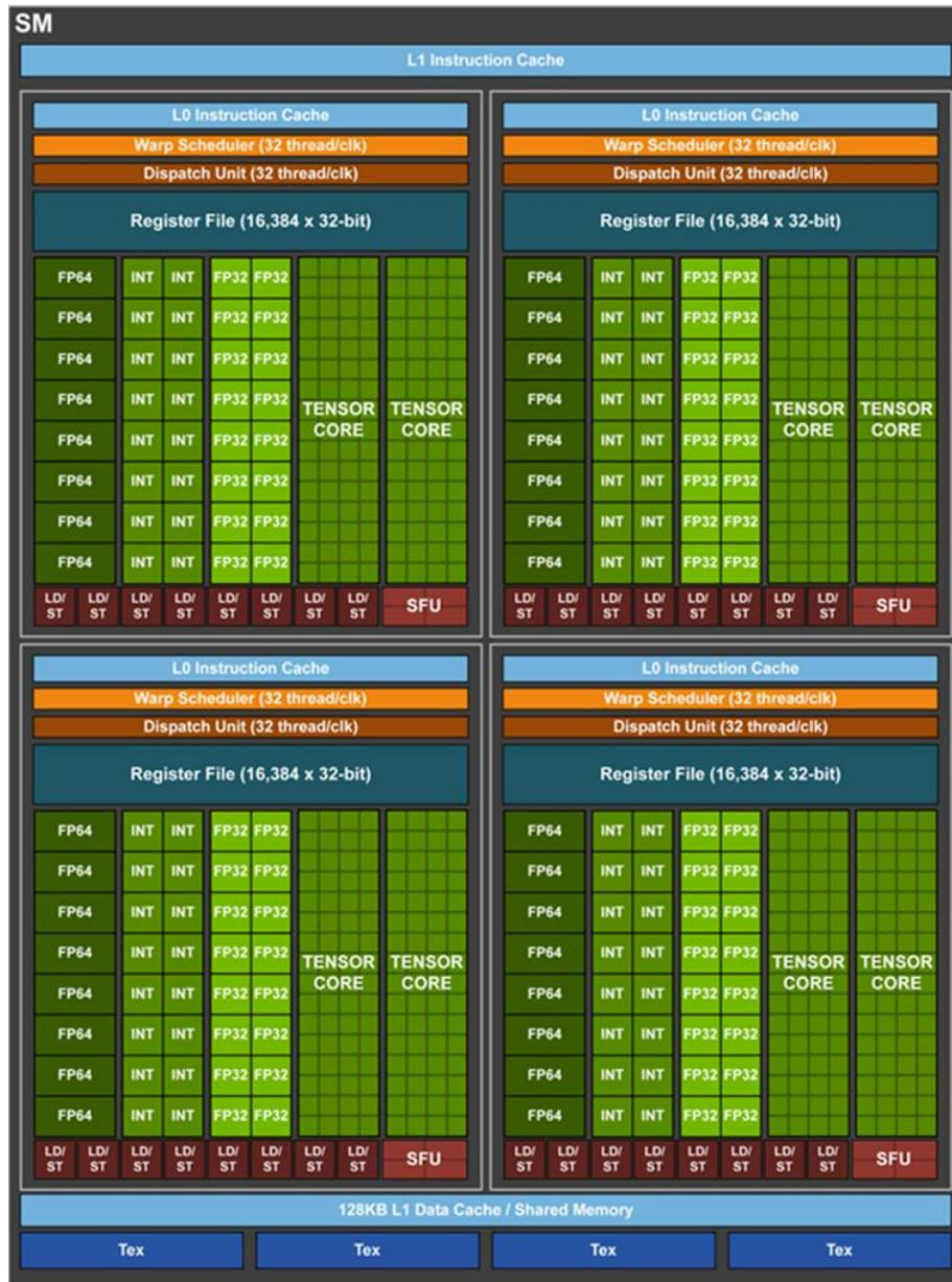
Figure 1.3: Architecture of streaming multi-processors in *NVIDIA*<sup>®</sup> Tesla V100 GPU [11].
