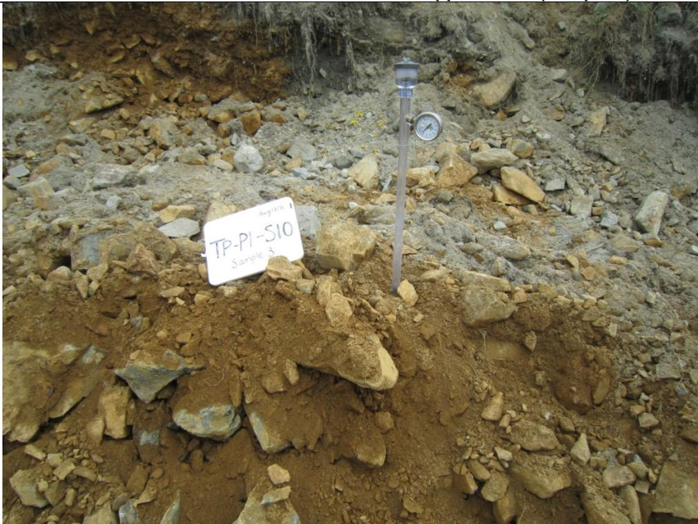
**Photo 4 – TP-P1-S10 waste rock excavated from test pit showing potassic alteration**
