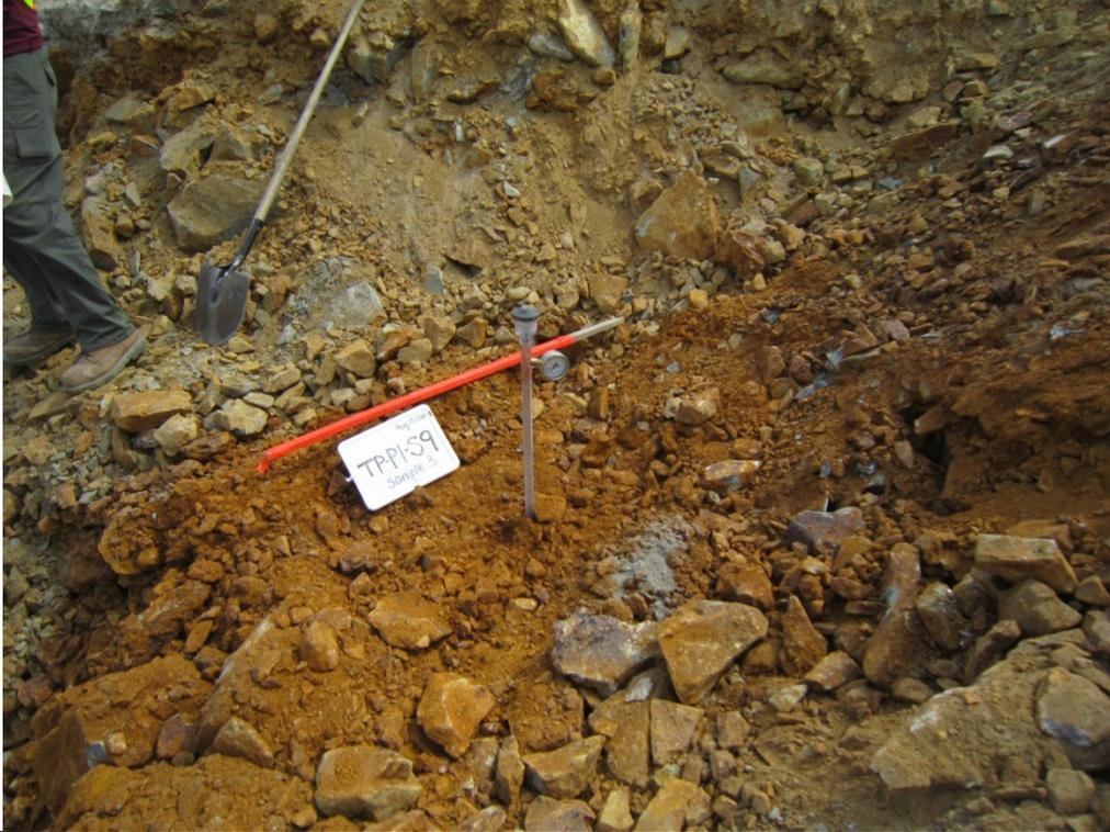
**Photo 4 – TP-P1-S9 waste rock excavated from test pit showing potassic alteration**
