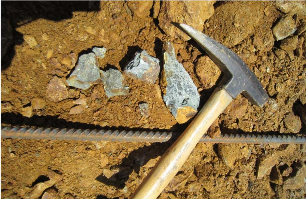
**Figure 3.6 - Location showing fresh surface of waste rock material with highly oxidized fine matrix and oxidation on surfaces of clasts.**
