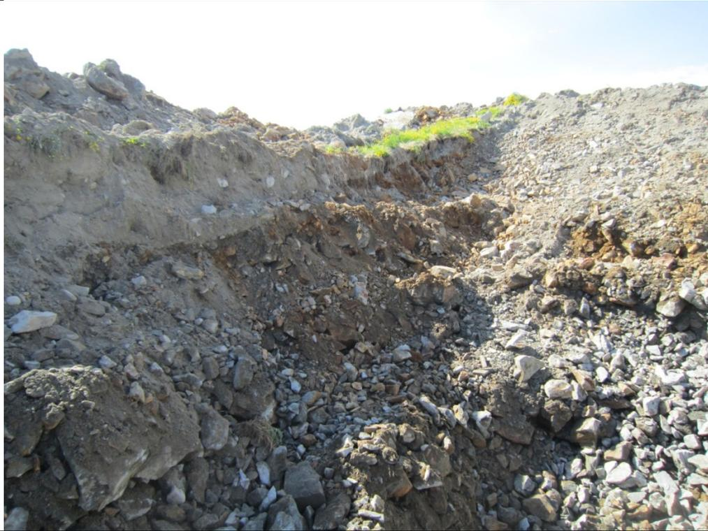
**Photo 4 – TP-P1-S14 waste rock excavated from test pit showing grain size range**
