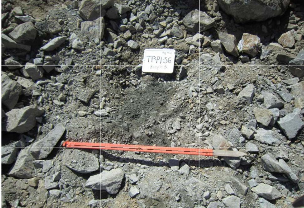
**Figure 5.1- Photo of sampling location TP-P1-S6-S3 using in DIP analysis prior to delineations with orange reference stake indicating 1 m**
