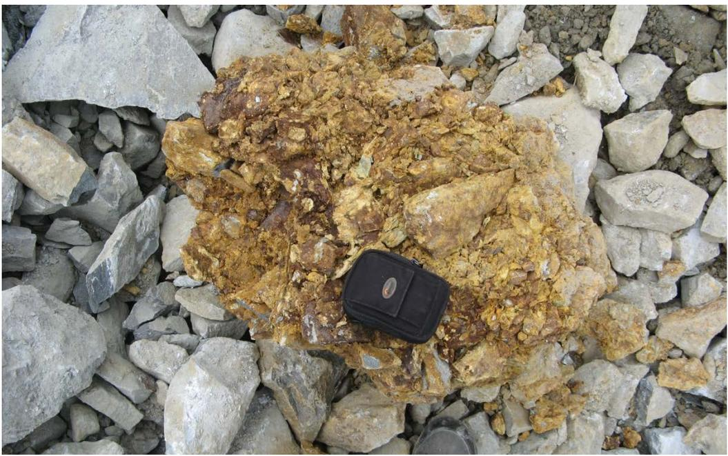
Figure 4.6 - Oxidation of waste rock on WRS 1 resulting in agglomeration and cementation of smaller particles
