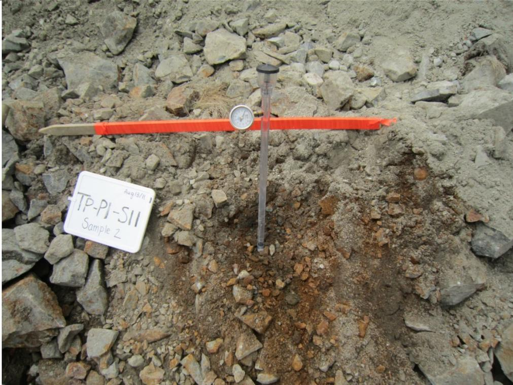
**Photo 3 – TP-P1-S11 tensiometer installation on upper bench (Sample 3)**
