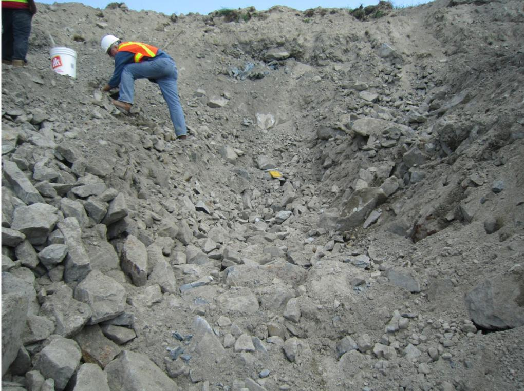
**Photo 4 – Grain size range found in test pit, some orange oxidation on particles surfaces**
