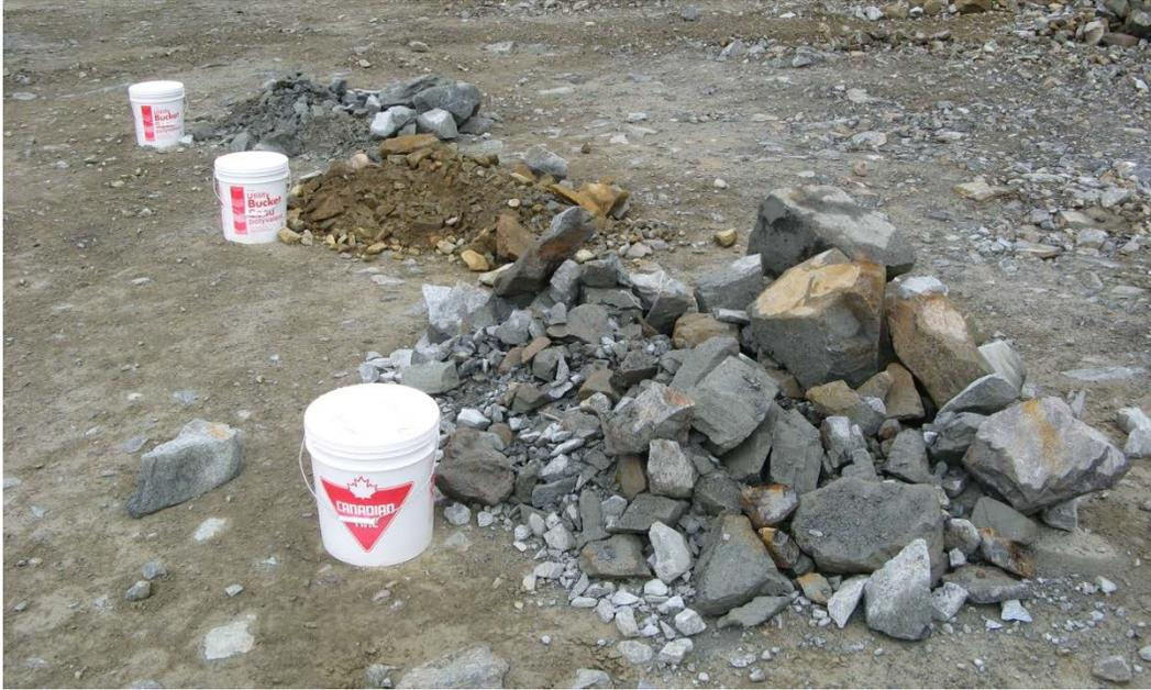
**Figure 3.10 – Material placed by an excavator from three sampling locations during the WRS 1 profile investigation. Subsamples were taken in 20-L plastic pails. Note differing waste rock sizes, textures, and colours.**
