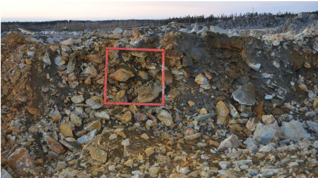
**Figure 3.8 – Typical excavated waste rock face on Waste Rock Stockpile 2 with a 1 m reference square**
