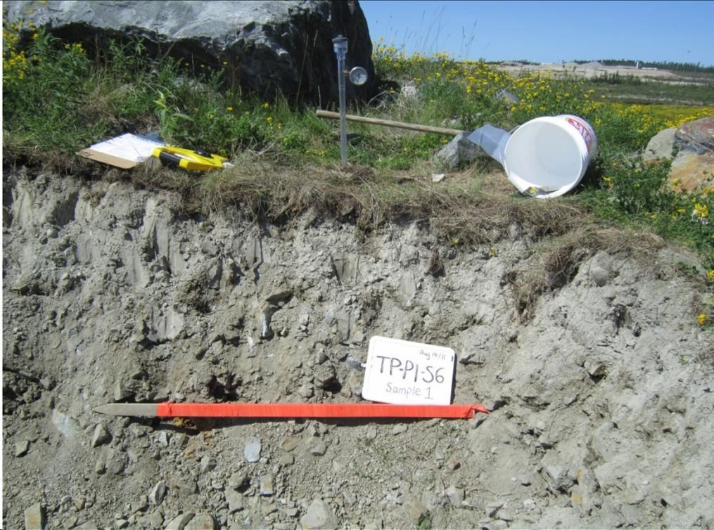
**Photo 4: TP-P1-S6 sampling location 2 showing oxidation of fines**
