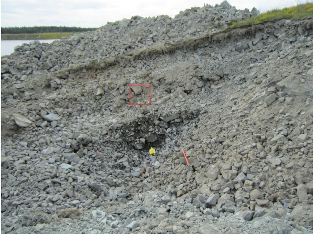
**Photo 3 – TP-P2-S12 bottom of test pit showing blocky gradation**
