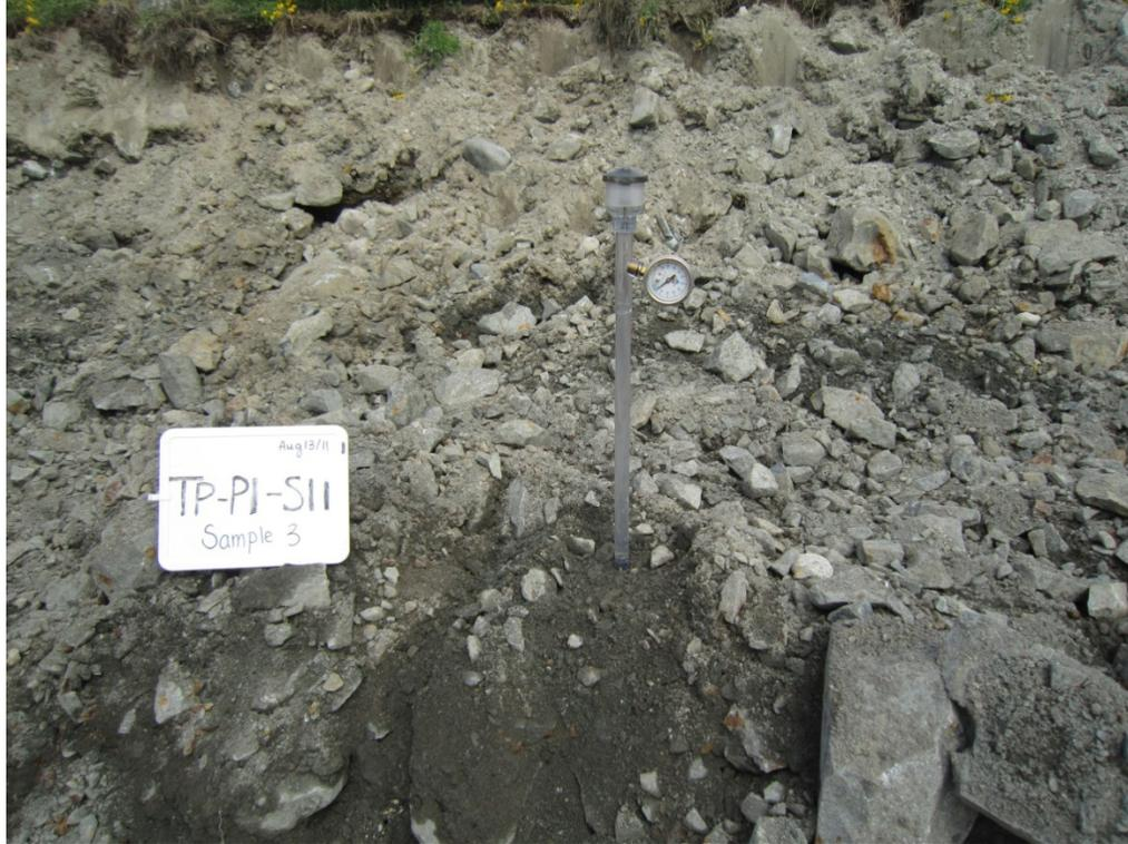
**Photo 4 – TP-P1-S11 waste rock excavated from test pit showing grain size range**
