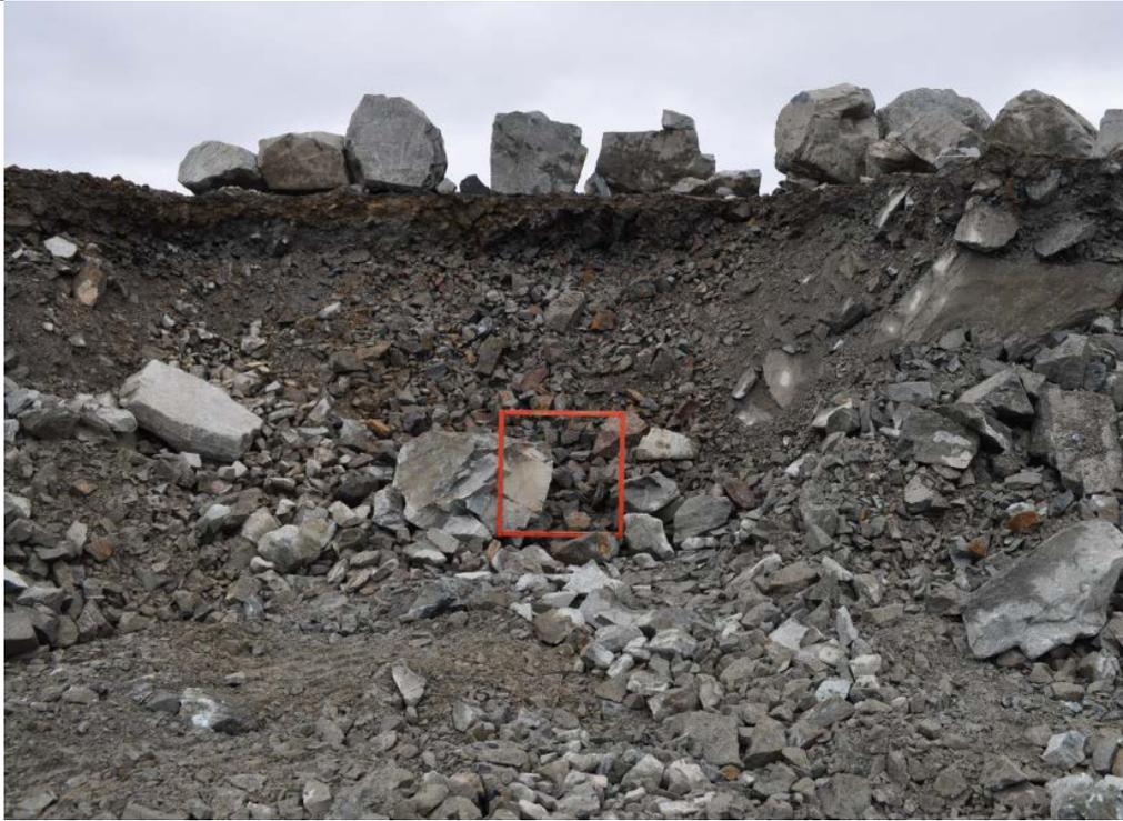
**Photo 2 – Sample after extraction by front end loader**
