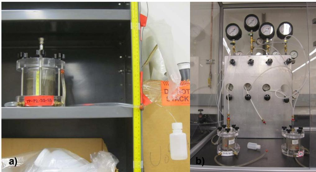
**Figure 3.16 – a) Hanging column testing method, b) Pressure regulator apparatus**
