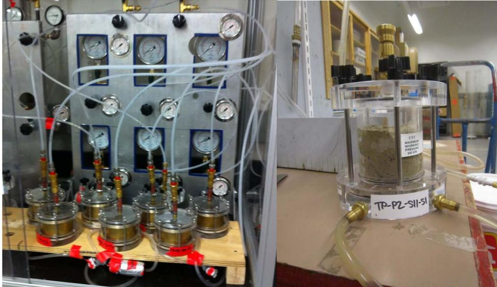
**Figure 3.15 - Typical Tempe cell pressure chamber**
