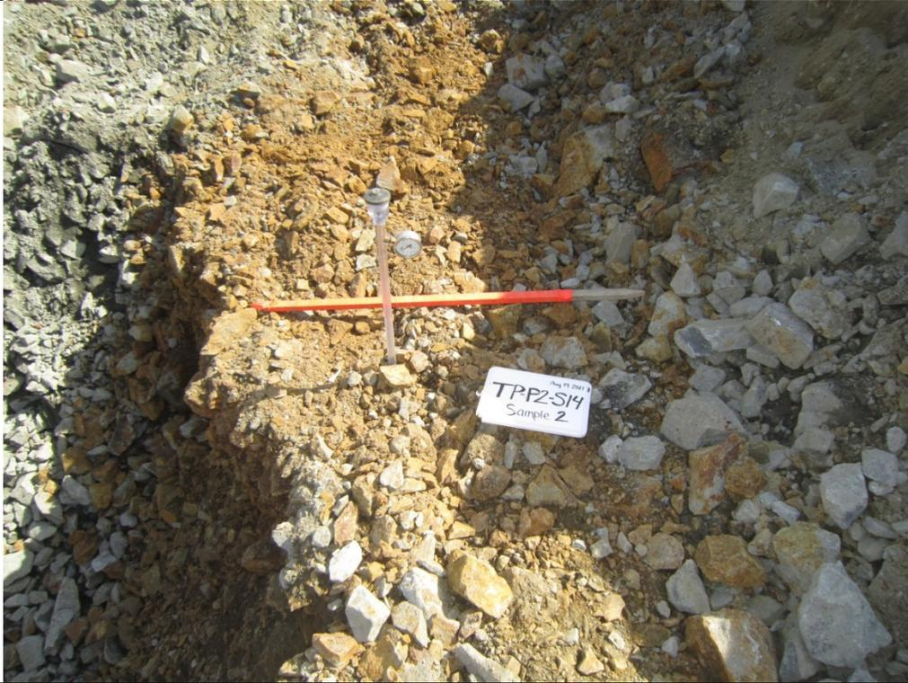
Photo 4 – TP-P2-S14 tensiometer installation in pit bottom (Sample 3)
