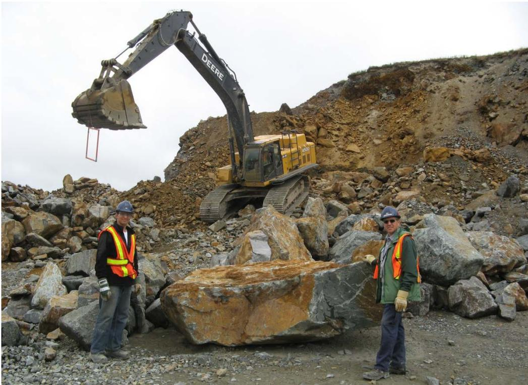
**Figure 3.11 - 20-L pail samples were limited to fine material. Grain size was observed in excess of 1 m.**
