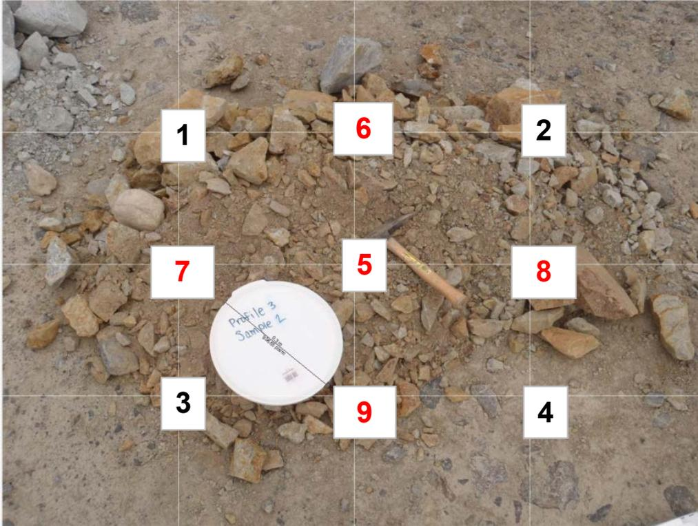
**Figure C.15 - Sampling location P1-P3-S2 with section numbers for the evaluation of the range of grain size using Split Desktop**
