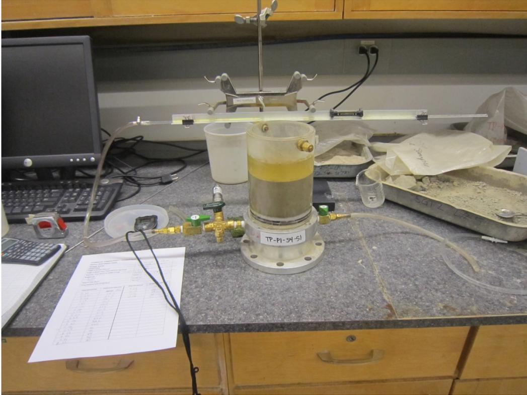
**Figure 3.14 - Setup of a typical constant head permeability test**
