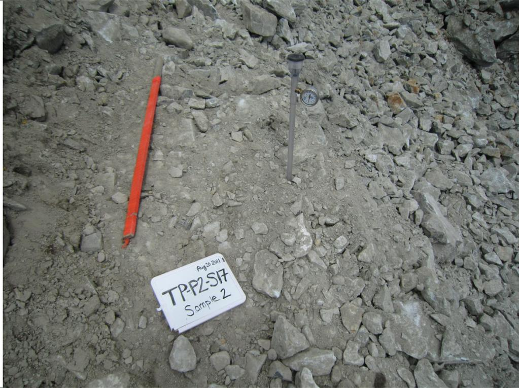
**Photo 4 - TP-P2-S17 base of test pit showing open voids and clast structure**
