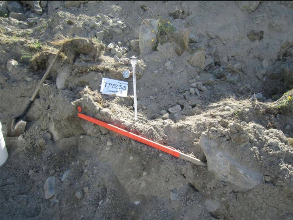
**Photo 3 – TP-P2-S13 test pit profile looking south showing tensiometer installations**
