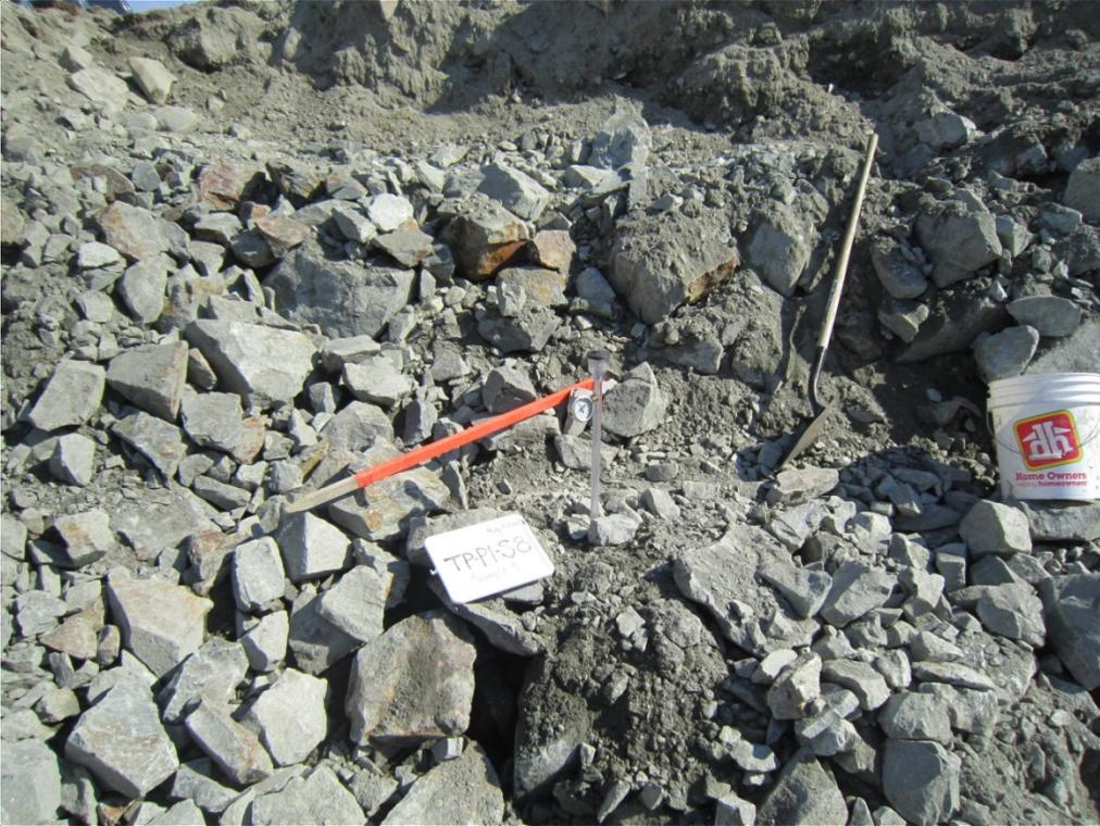
**Photo 4: TP-P1-S8 waste rock excavated from test pit showing grain size range**
