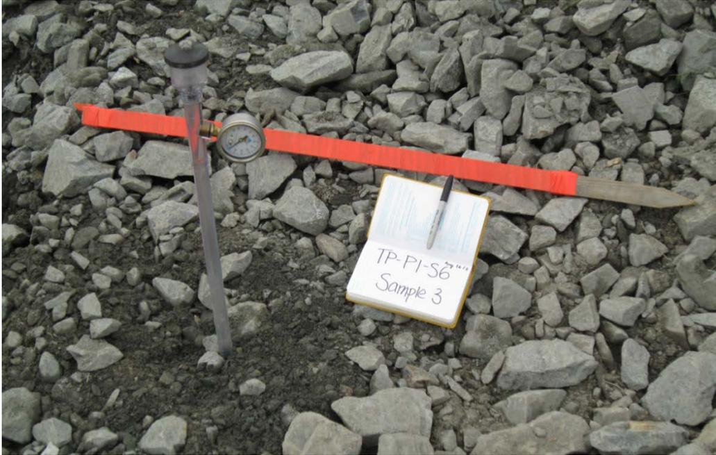
**Figure 3.4 - Typical tensiometer installation in fine material.**
