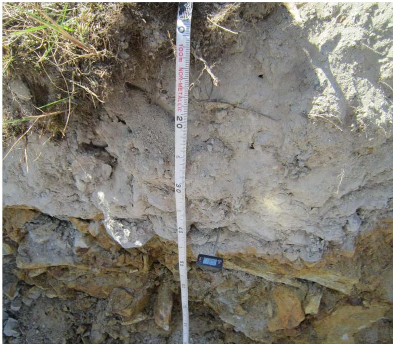
**Figure 3.5 – Measurement of soil and waste rock temperature in a test pit wall**
