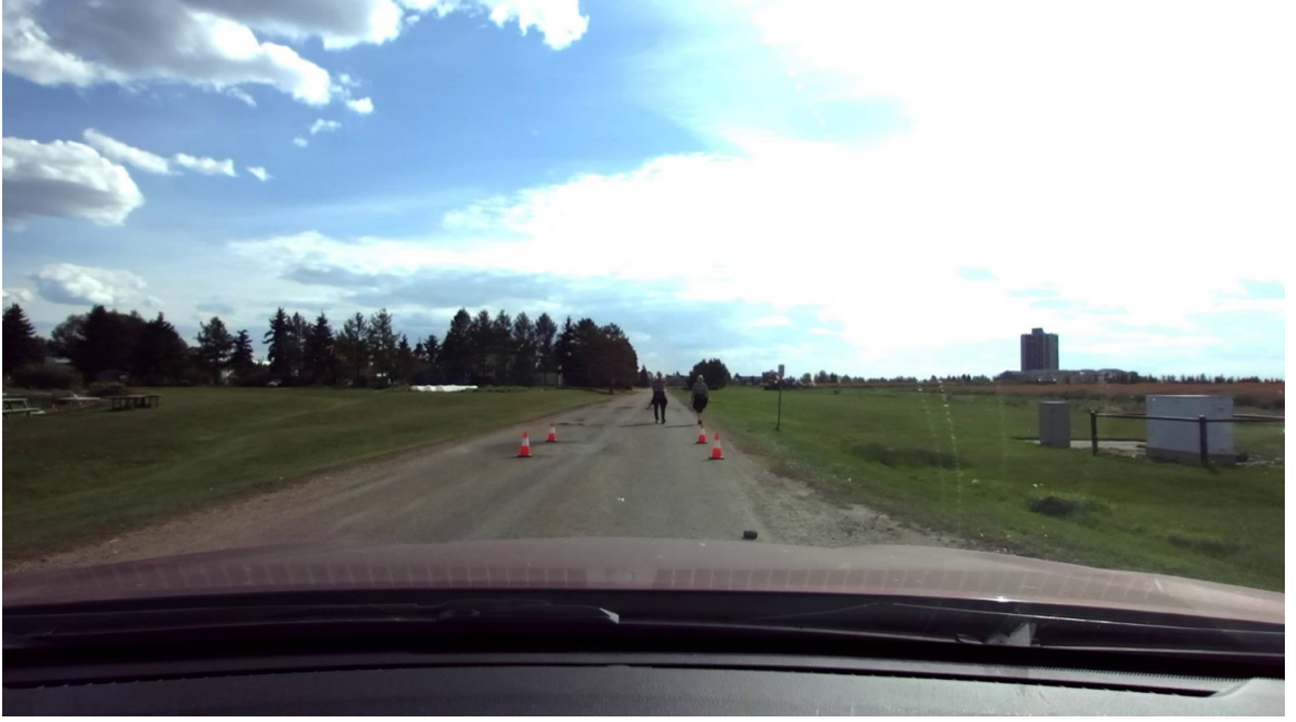
Figure 4.4: cones are arranged in a 7.5 meter by 7.5 meter square, located 15 meters ahead of the vehicle.
