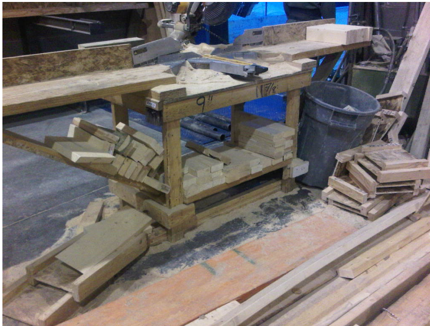
Figure 5-19: Saw Table at Floor Prefab Cell (Before 5S)
