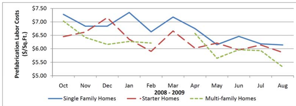
Figure 5-18: Average Labor Costs of GC Prefabrication
