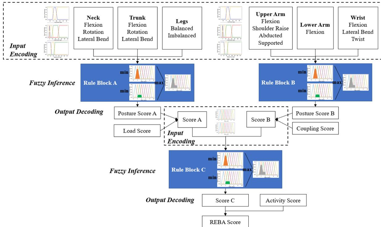
Figure 4-2. Rule-based fuzzy inference algorithm in REBA
