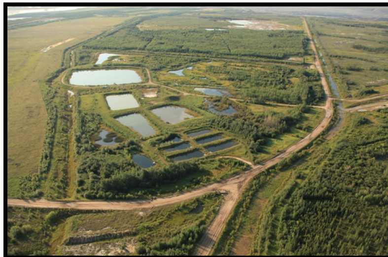
Figure 6: Ponds utilized by Syncrude over the last two decades to test water capping technology (Syncrude, 2012)
