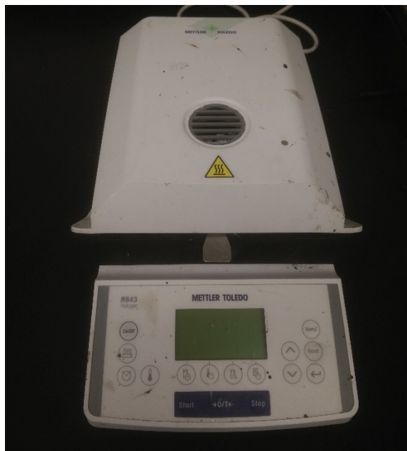
Figure 47: Mettler Toledo HB43-S Halogen Moisture Analyzer
