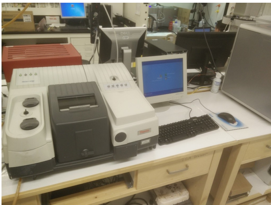
Figure 46: Thermo Nicolet 6700 Fourier Transform Infrared (FTIR) spectrometer
