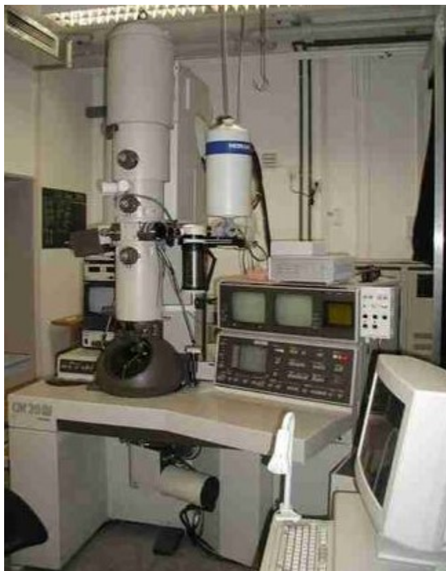
Figure 48: Philips CM20 FEG TEM/STEM transmission electron microscope (IFW, 2015)
