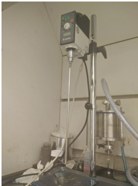
Figure 45: Heidolph™ Electronic Overhead Stirrer (RZR 2052 Control)
