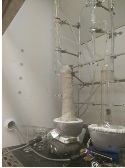
Figure 43: Dean Stark extraction set up for determining bitumen, water and solids content
