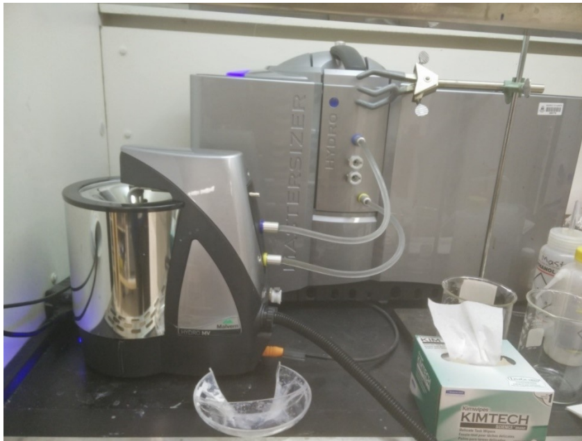
Figure 42: Mastersizer 3000 used for laser particle size analysis
