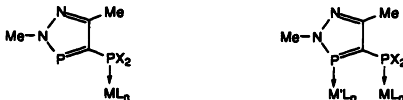
Figure 4.1 Monodentate coordination and bridging action of the phosphino-2,5-dimethyl-2 H -1,2,3σ 2 -diazaphospholes with metal centres.
