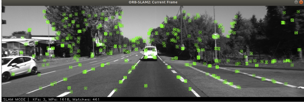
Figure 2.6: A visualization of ORB-SLAM2 during execution of a Stereo sequence. The green circles represent the ORB features that are being created and matched.
