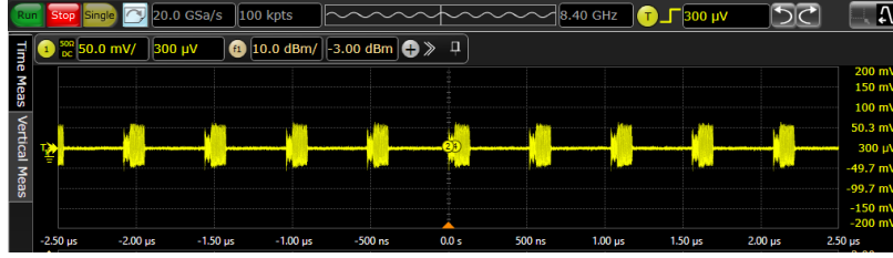
Figure 5.21: Chip output waveform when V_{IN1} = 0 , V_{IN2} = 0 , V_{DD} = 600mV , and I_{REF} = 1.5 \mu A .
