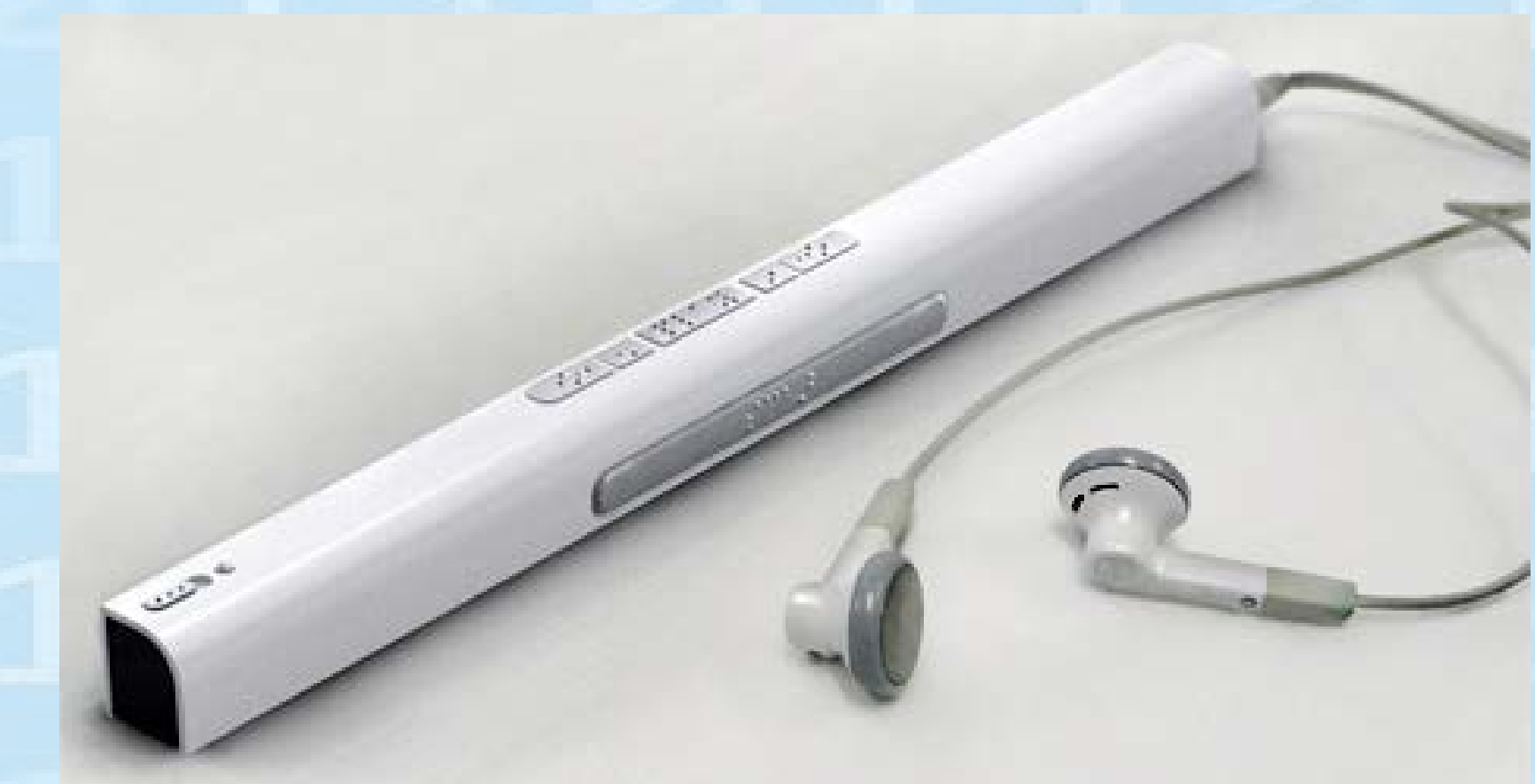
Figure 13: Portable voice stick made with OCR to instantly translate text to audio for the visually impaired (Park).
