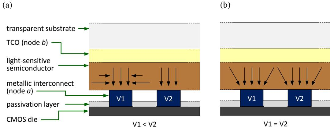
Figure 4.2: Cross section of the structure shown in Fig. 4.1. (a) When the light-sensitive semiconductor layer is unpatterned, potential differences between adjacent pixels results in flow of lateral currents toward pixels with lower potentials. (b) Lateral currents can be reduced by maintenance of a constant potential at all pixels. The electric field needs to be strong enough to overcome diffusion of charge carriers due to concentration gradients.
