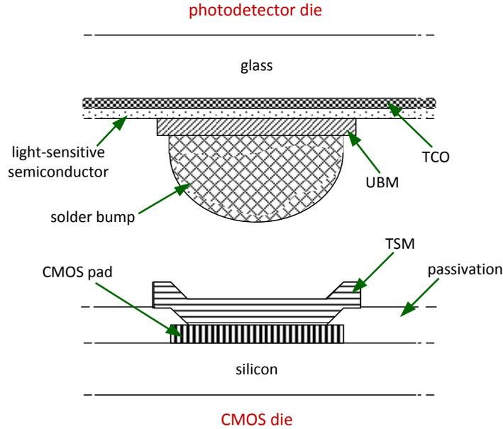
Figure 3.4: Pre-processing required for flip-chip bonding (not drawn to scale). TSM is deposited on the CMOS die, and UBM is deposited on the photodetector die. Solder bumps, tens of microns thick, are fabricated on the UBM.
