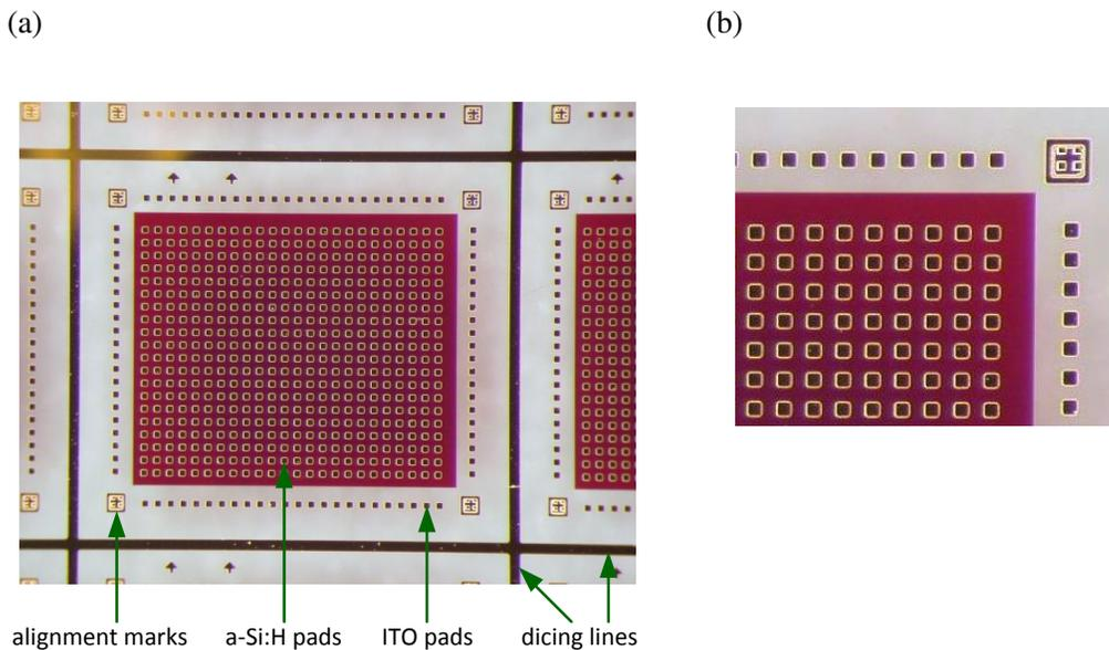
Figure A.6: (a) Photodetector dies with photodetectors for a prototype VI-CMOS image sensor. (b) A closer look at a photodetector array. Bond pads, i.e., the UBM for flip-chip bonding, are visible on the a-Si:H and ITO regions.
