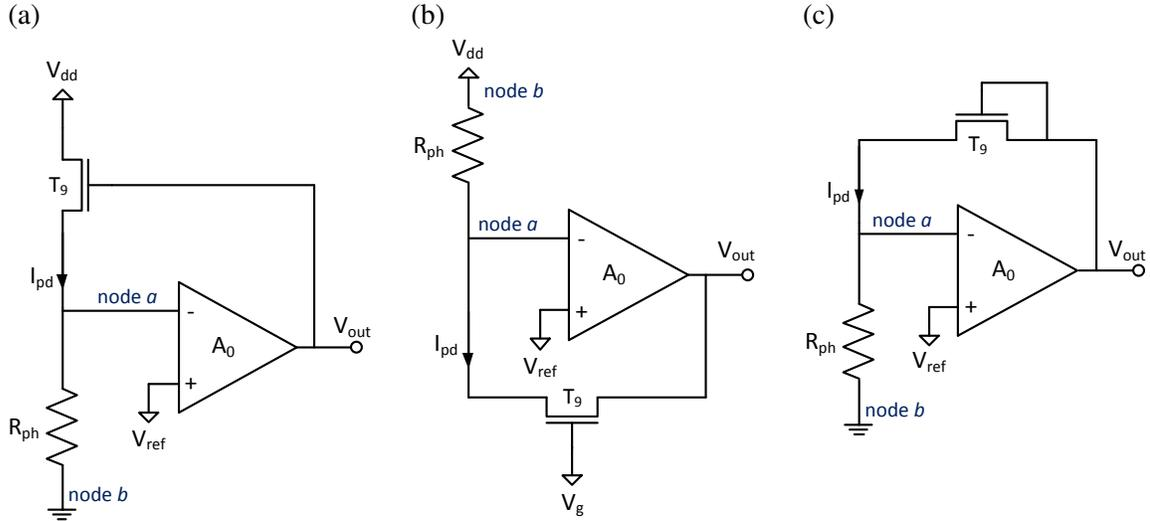
Figure 4.5: A logarithmic response can be achieved by placing a MOS transistor, which operates in the sub-threshold region, in the feedback loop. This work considers three optional configurations: (a) the common-drain, (b) the common-gate, and (c) the “diode-connected” transistor.
