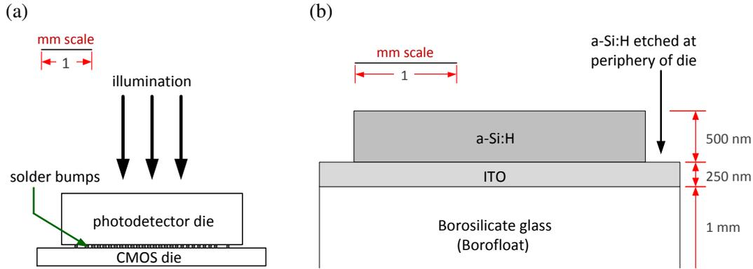
Figure A.1: (a) The VI-CMOS image sensor prototype is composed of a CMOS die and a photodetector die. It is assembled by flip-chip bonding. (b) To prepare the photodetector die, ITO is deposited on a borosilicate glass substrate, and a-Si:H film is deposited on the ITO and then etched from the periphery. To enable flip-chip bonding to the CMOS die, bond pads need to be formed on the a-Si:H and ITO regions.
