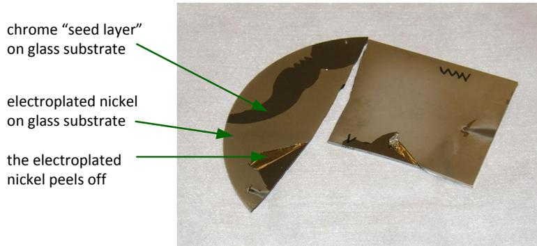
Figure A.3: In an early electroplating trial, we electroplated nickel onto glass substrates that were coated with sputtered chrome. Although the chrome had a good adhesion to the glass, it proved to be an unsuitable seed layer for the electroplated nickel. In the photo, one can see that the nickel layer peels off easily.
