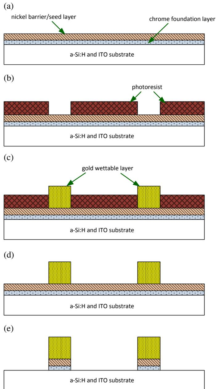
Figure A.4: Fabrication of bond pads: (a) Sputtering of a 100 nm foundation layer of chrome and a 200 nm barrier/seed layer of nickel. (b) Lithography—only the areas that will be bond pads are exposed. (c) Electroplating of a 1.5  $\mu\text{m}$  wettable layer of gold. Deposition occurs only on the exposed nickel, which is connected to the cathode. (d) Stripping of the photoresist. (e) Etching of the nickel and chrome, except from underneath the gold.
