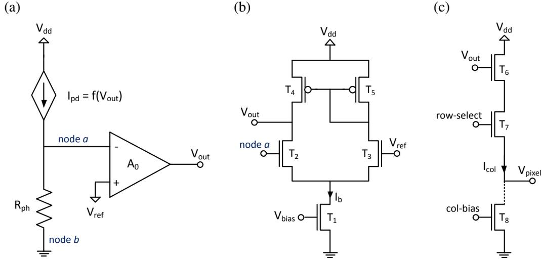
Figure 4.4: (a) Schematic of a feedback active pixel. A constant potential,  $V_{ref}$ , is maintained at node  $a$  using an op-amp with a negative feedback loop. A voltage-controlled current source (VCCS) generates a current,  $I_{pd}$ , that varies as a function of  $V_{out}$ . (b) The amplifier may be implemented using a differential-input op-amp with an active current-mirror load. (c) The output stage of the pixel circuit.
