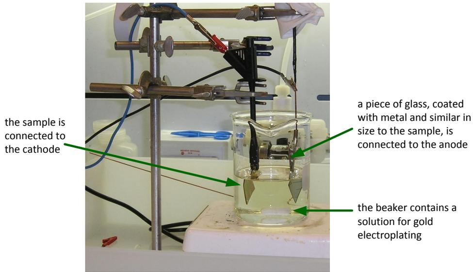
Figure A.5: The gold electroplating station: A beaker filled with a gold electroplating solution is placed on a hot plate that also provides stirring. The solution is heated to about 40 °C. The sample, on which the gold is to be deposited, is connected to the cathode. A comparable piece of glass with a conductive coating is connected to the anode. A power supply keeps a constant current between the electrodes while monitoring the voltage.
