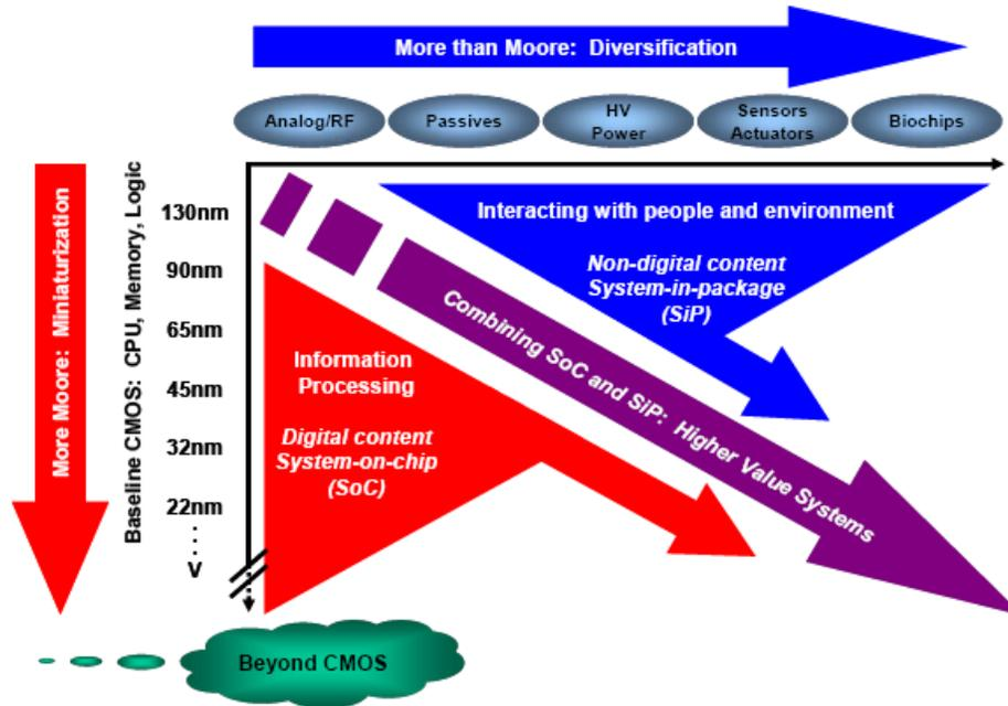
Figure 1.1: Diagram taken from a white paper of the ITRS that was released in 2010 [13]. The dual trend of the ITRS includes device miniaturization, or “More Moore”, as well as functional diversification, or “More than Moore”.
