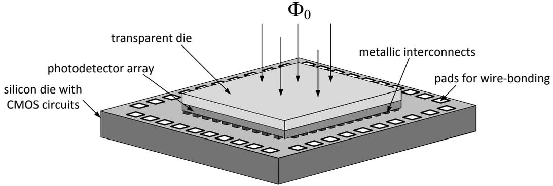
Figure 5.1: Schematic of a VI-CMOS image sensor fabricated by flip-chip bonding. A transparent die with an array of photodetectors is bonded through metallic interconnects to an array of readout circuits on a CMOS die. The CMOS die, which is prepared in a standard CMOS process, also contains peripheral circuits and bond pads for external communication.  $\Phi_0$  refers to the incident illumination.
