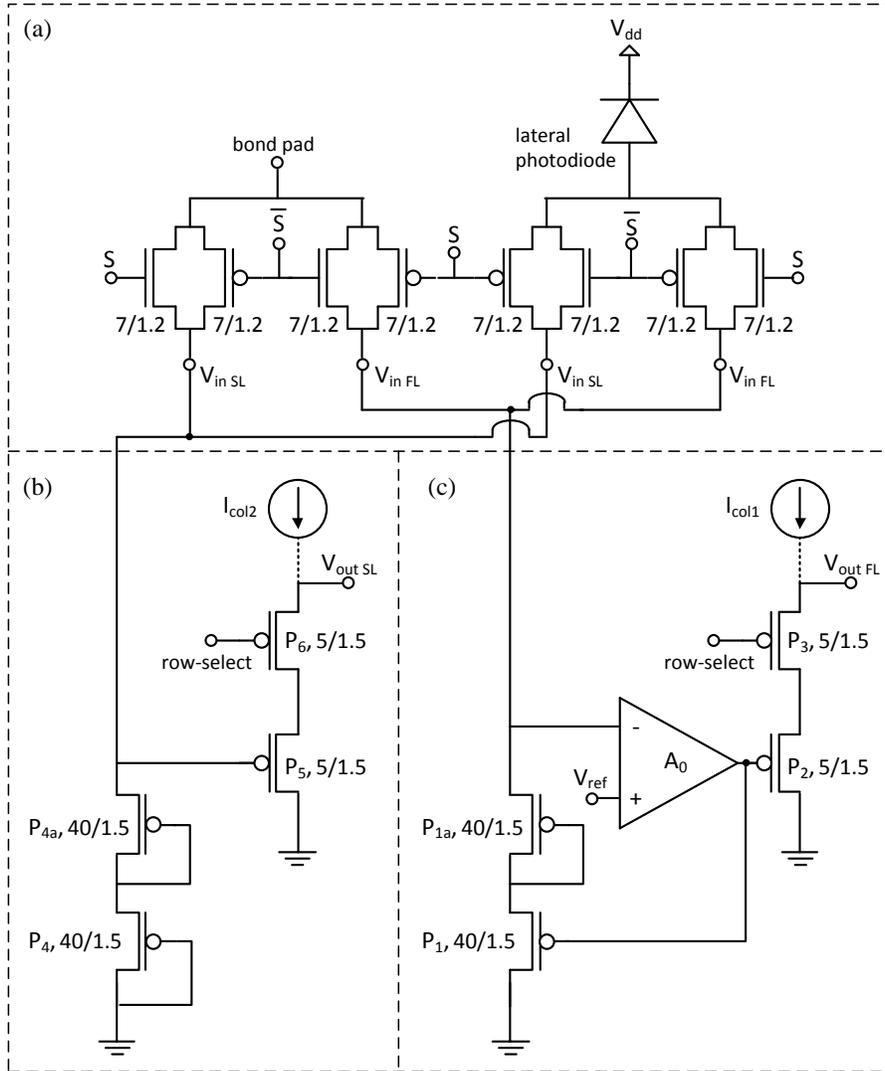
Figure 3.6: Principal schematics of the active pixel: (a) the switch (SW); (b) the standard logarithmic-response (SL) circuit; and (c) the feedback logarithmic-response (FL) circuit. The control signal  $S$  configures transmission gates connected to a bond pad (BP), which is used for integration with a vertical photodetector, and to a lateral photodiode (LP).
