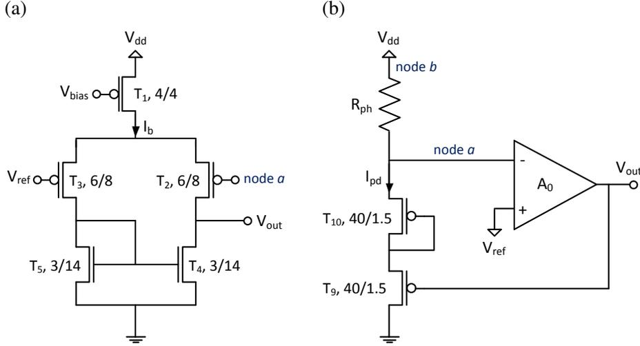
Figure 4.7: Schematics of (a) the op-amp and (b) the entire feedback active pixel. These circuits were used for simulations and were implemented in the CMOS die of a fabricated VI-CMOS prototype.
