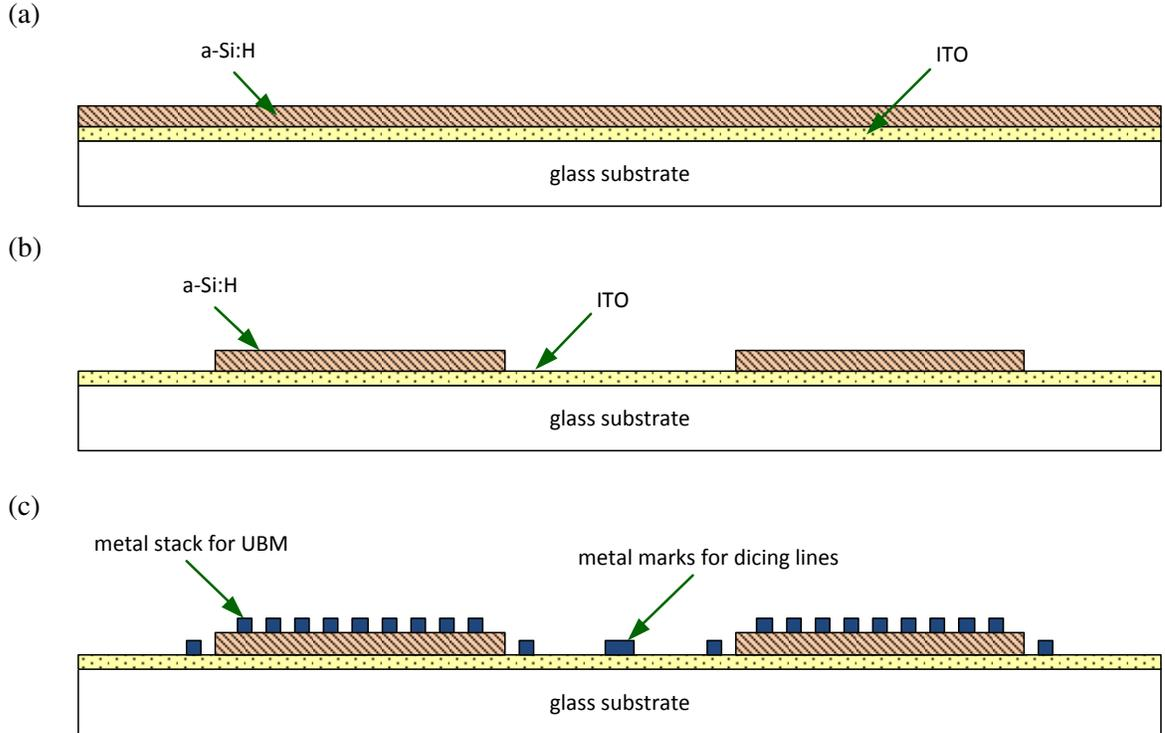
Figure 3.8: Fabrication process of the designed photodetector die. (a) ITO is sputter deposited and then annealed. An a-Si:H film is deposited by PECVD on the ITO. (b) The first lithography step uses reactive ion etching to expose ITO at the periphery of a-Si:H rectangles. (c) An array of bond pads is formed on the a-Si:H rectangles, with further bond pads on the surrounding ITO. A metal grid is deposited with the bond pads to mark dicing lines on the coated glass substrate.
