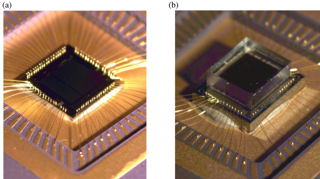
Figure 3.1: (a) CMOS and (b) VI-CMOS image sensors designed at the University of Alberta and fabricated via CMC Microsystems. With the CMOS sensor, each pixel includes a photodetector integrated laterally with CMOS transistors. With the VI-CMOS sensor, a CMOS die (bottom), which includes an active pixel sensor array, is vertically integrated with a photodetector die (top), which includes a photodetector array fabricated on a glass substrate.
