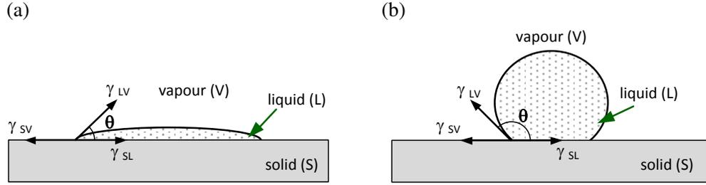
Figure A.2: (a) When  $\theta < 90^\circ$ , the surface is wetted by the liquid. (b) When  $90^\circ < \theta < 180^\circ$ , the liquid does not spread on the surface. Formation of a thin oxide layer on a metal surface reduces the surface free energy. The small  $\gamma_{SV}$  forces large  $\theta$ , and this prevents molten solder from wetting the oxidized surface.
