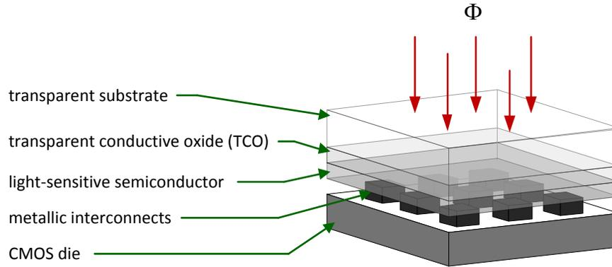
Figure 4.1: Central area of a VI-CMOS image sensor. The CMOS die also contains peripheral circuits and bond pads for wire bonding, which are intended for communication with the external world.  $\Phi$  refers to the incident illuminance. The TCO layer is connected to a constant potential supplied through the CMOS die by peripheral metallic interconnects (not shown).
