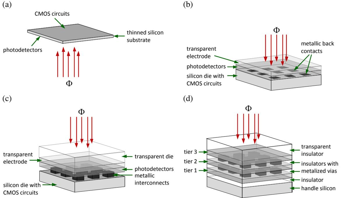
Figure 3.2: VI-CMOS image sensors fabricated by (a) thinned substrate, (b) thin-film-on-ASIC (TFA), (c) flip-chip, and (d) through-substrate via (TSV) technologies.
