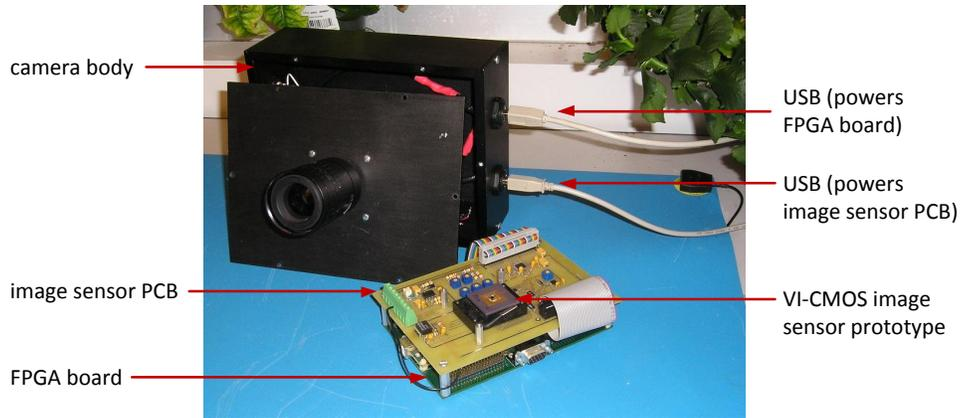
Figure 3.11: Digital camera that was designed and built to test the VI-CMOS prototype. The camera body accommodates a commercial board with an FPGA and a custom-made board that includes the image sensor. Board powering and data transfer between the FPGA and a PC are done through two USB ports.
