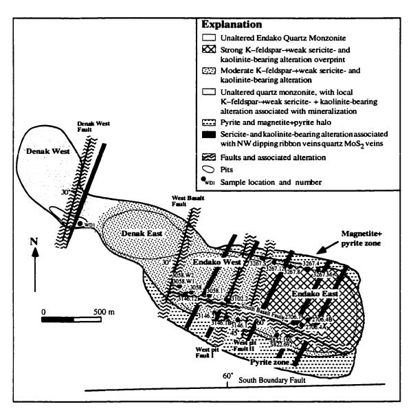
Fig. 2.3. Hydrothermal alteration map of the Endako deposit, with locations of samples analyzed for fluid inclusion studies.
