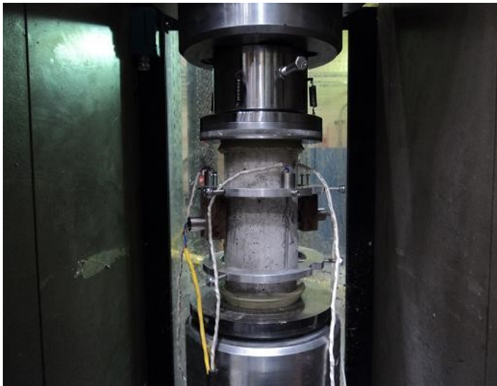
Figure 7-2: Compression test setup
