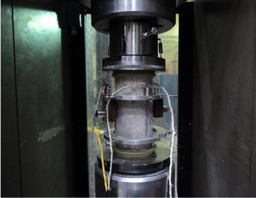
Figure 4-1: Test setup for quasi static compression testing
