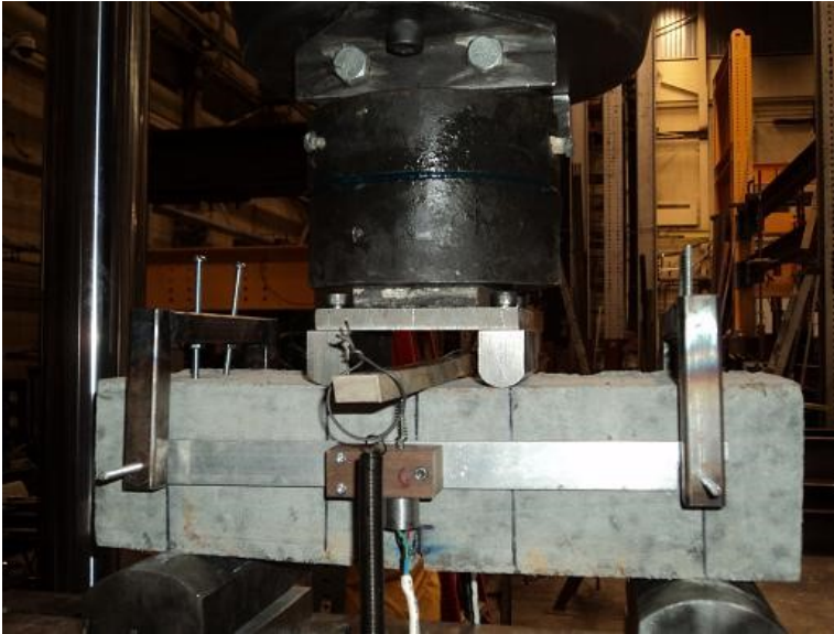
Figure 7-3: Quasi static flexural test setup
