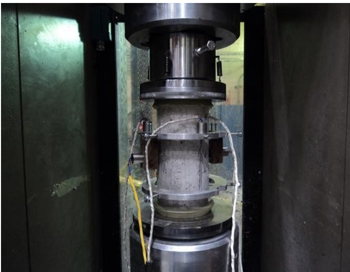
Figure 3-3: Compression test setup
