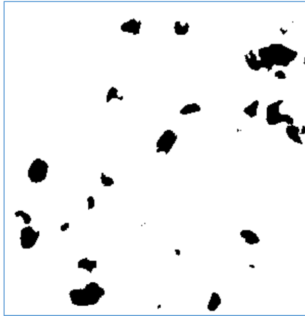
Figure IV-1: Sample image analysis of FRP bar surface (16 mm)
