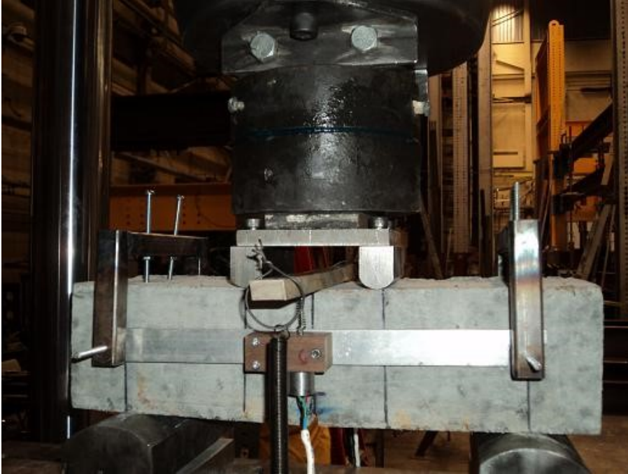
Figure 3-4: Quasi-static flexural test setup
