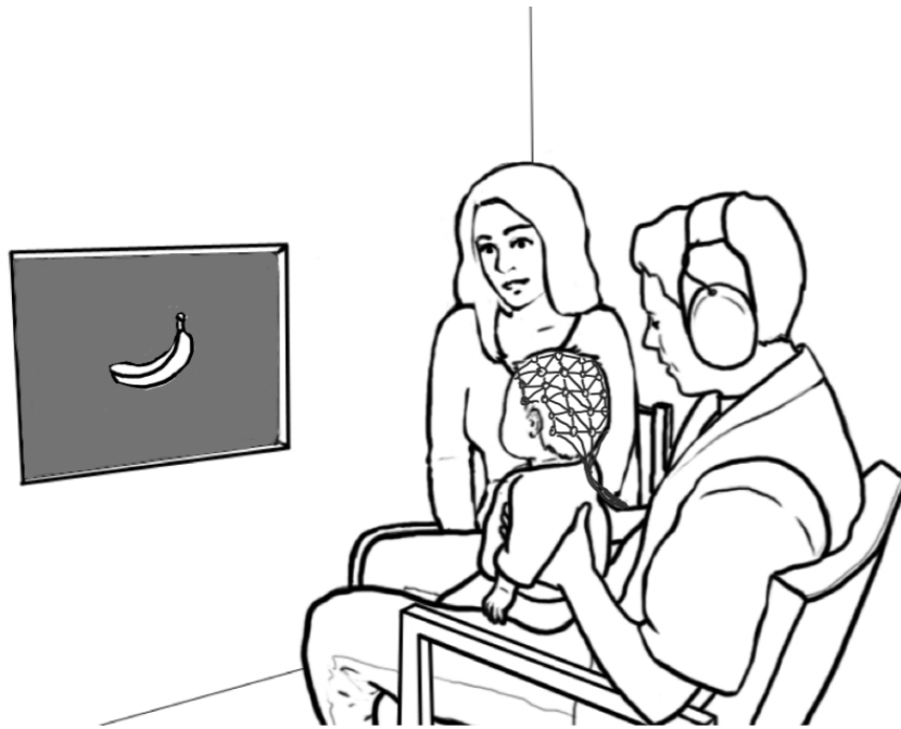
Figure 3.3: Experimental room setup where the data was collected. The participants sat on their parent's lap and the experimenter provided the word stimuli. Following the word stimuli, an image was shown on the screen placed in front of the participant.
