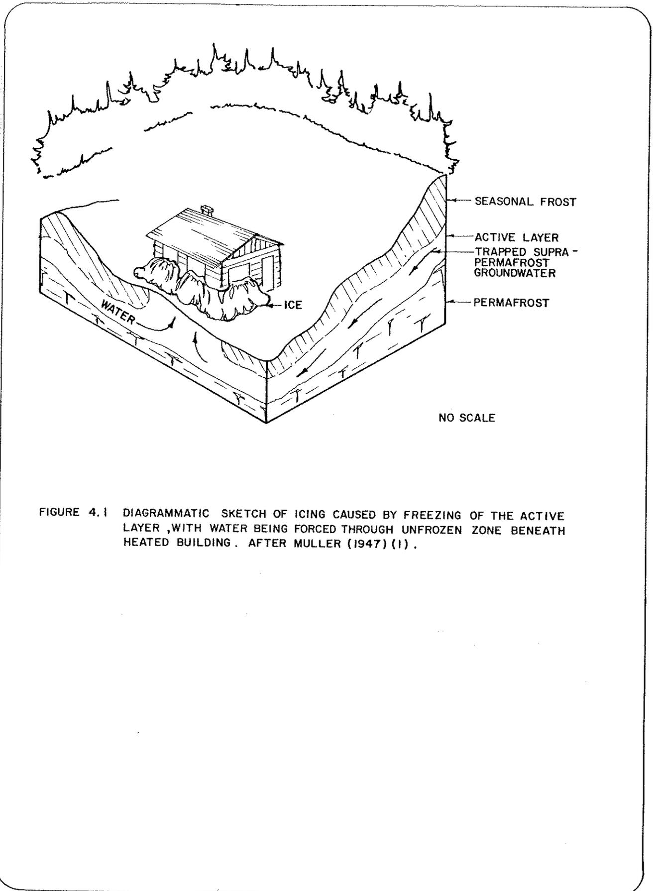
FIGURE 4.1 DIAGRAMMATIC SKETCH OF ICING CAUSED BY FREEZING OF THE ACTIVE LAYER ,WITH WATER BEING FORCED THROUGH UNFROZEN ZONE BENEATH HEATED BUILDING . AFTER MULLER (1947) (1) .
