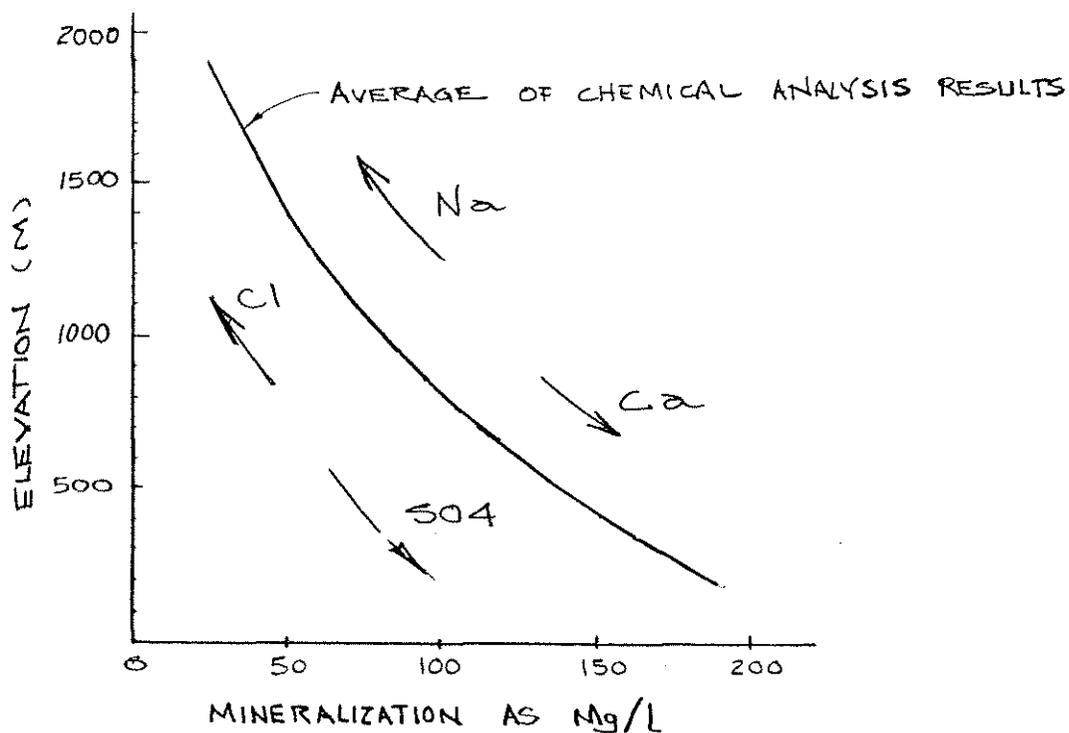
Figure 3.1. Changes in mineralization and composition of groundwater with elevation, after Tolstikhin (1974) (5).
