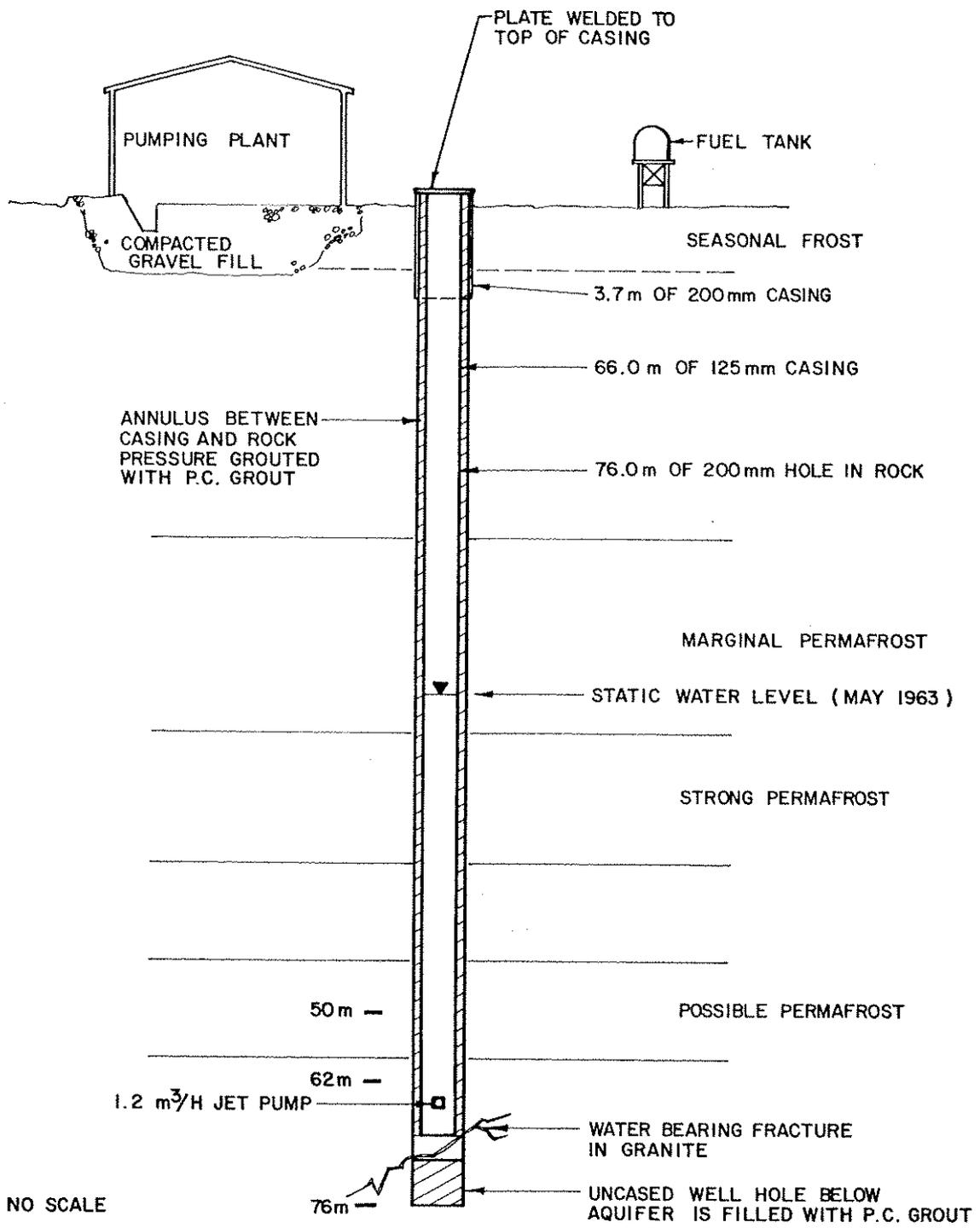
FIGURE 5.3 DIAGRAMMATIC SKETCH OF WELL IN GRANITE ( AT NORTHWAY , ALASKA ). FROM W. GEORGE (42) .
