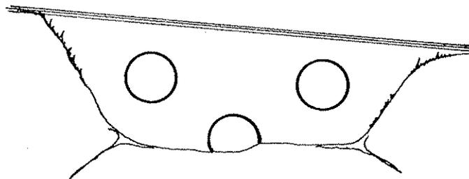
FIGURE 5.6 STAGGERED CULVERTS IN ROAD EMBANKMENT TO PASS SPRING RUNOFF .
