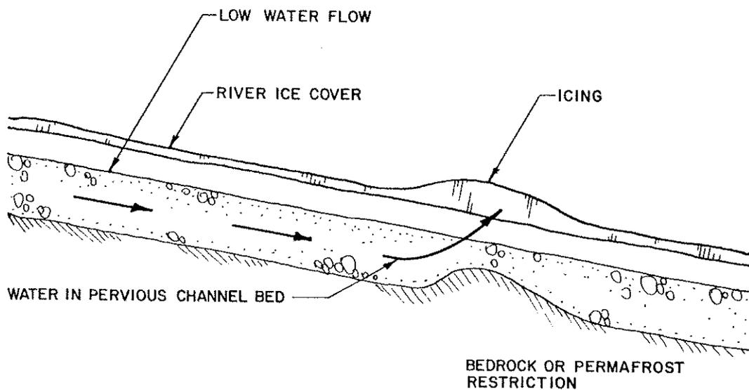
(a) RIVER ICING FORMED DUE TO OBSTRUCTION OF FLOW IN STREAM BED .
