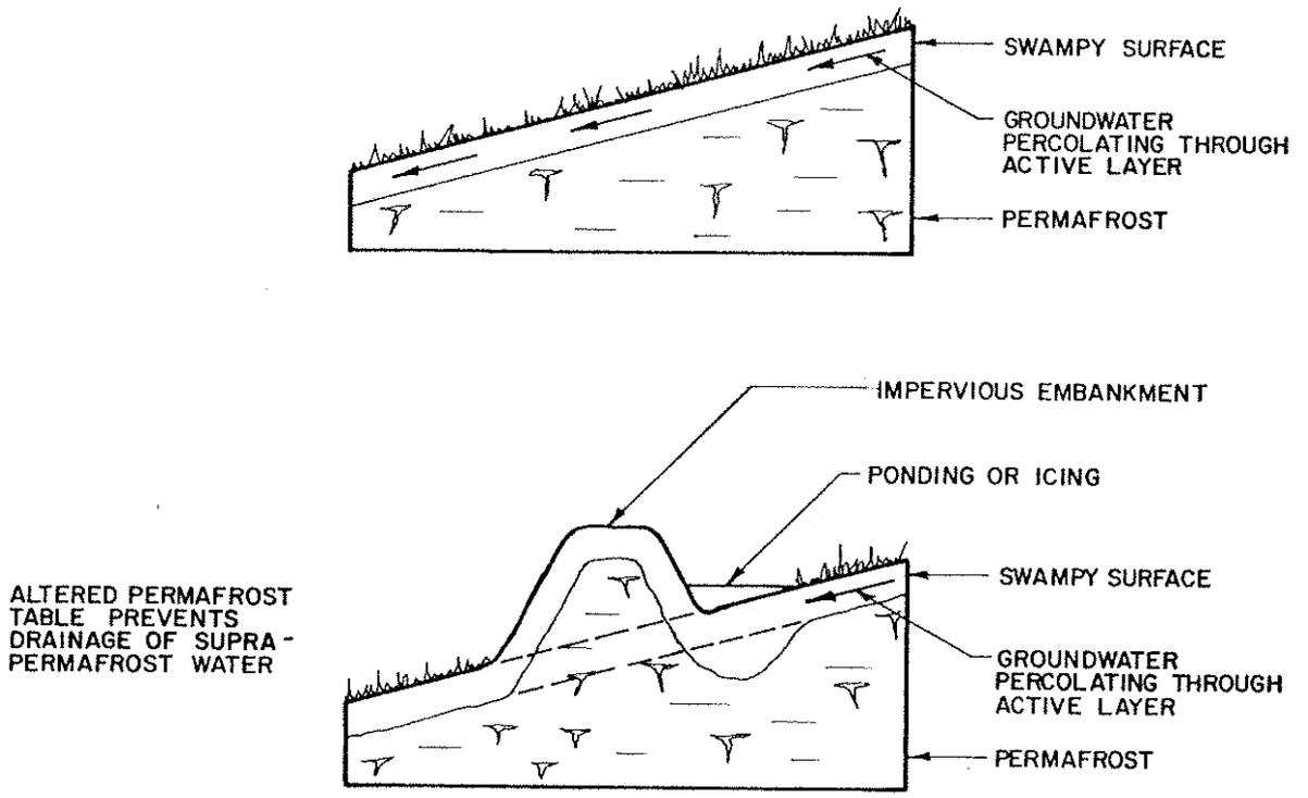
FIGURE 5.5 FORMATION OF AN ICING OR PONDING DUE TO DISTURBANCE OF THE ACTIVE LAYER BY EMBANKMENT CONSTRUCTION .
