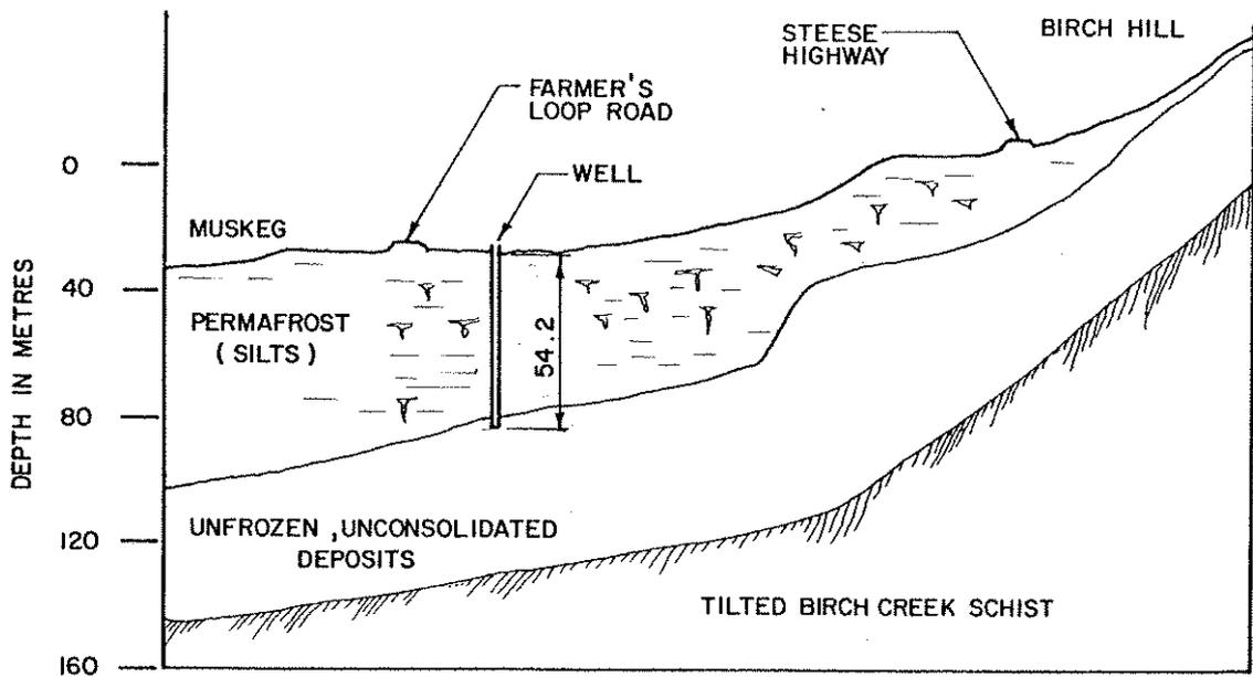
FIGURE 5.2 CROSS SECTION OF ARTESIAN SUBPERMAFROST AQUIFER NEAR FAIRBANKS , ALASKA .
