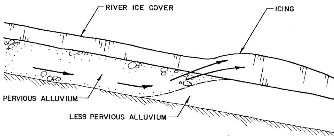
(b) RIVER ICING CAUSED BY CHANGE IN PERMEABILITY OF SUB - BED ALLUVIUM .
