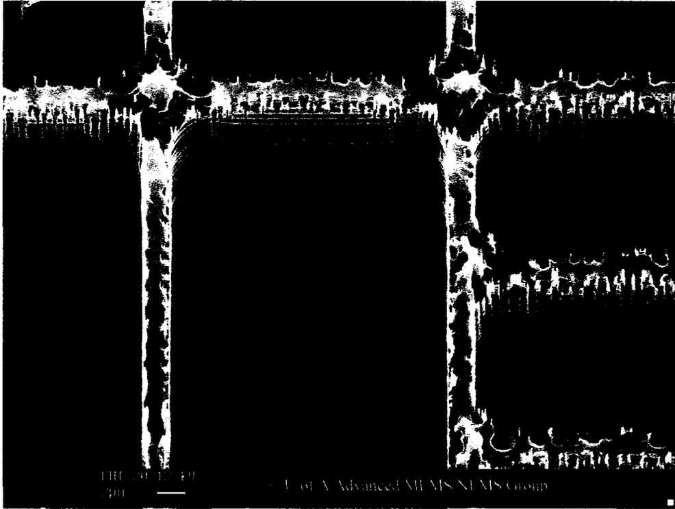
Figure 3.6: The tops of the lattice structures that lost their masking oxide and were etched during the DRIE process step.
